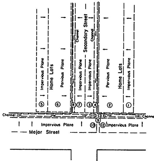
FIG. 5.—Geometric Segments for Typical Block in Urban Watershed
