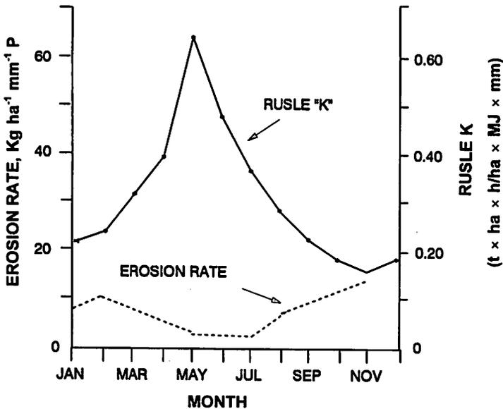
Fig. 5-9. Monthly measured erosion rate per millimeter of precipitation for the wet soil moisture condition on the clipped plots of the 1991 to 1992 Bernardino study and the RUSLE estimated monthly  $K$ .
