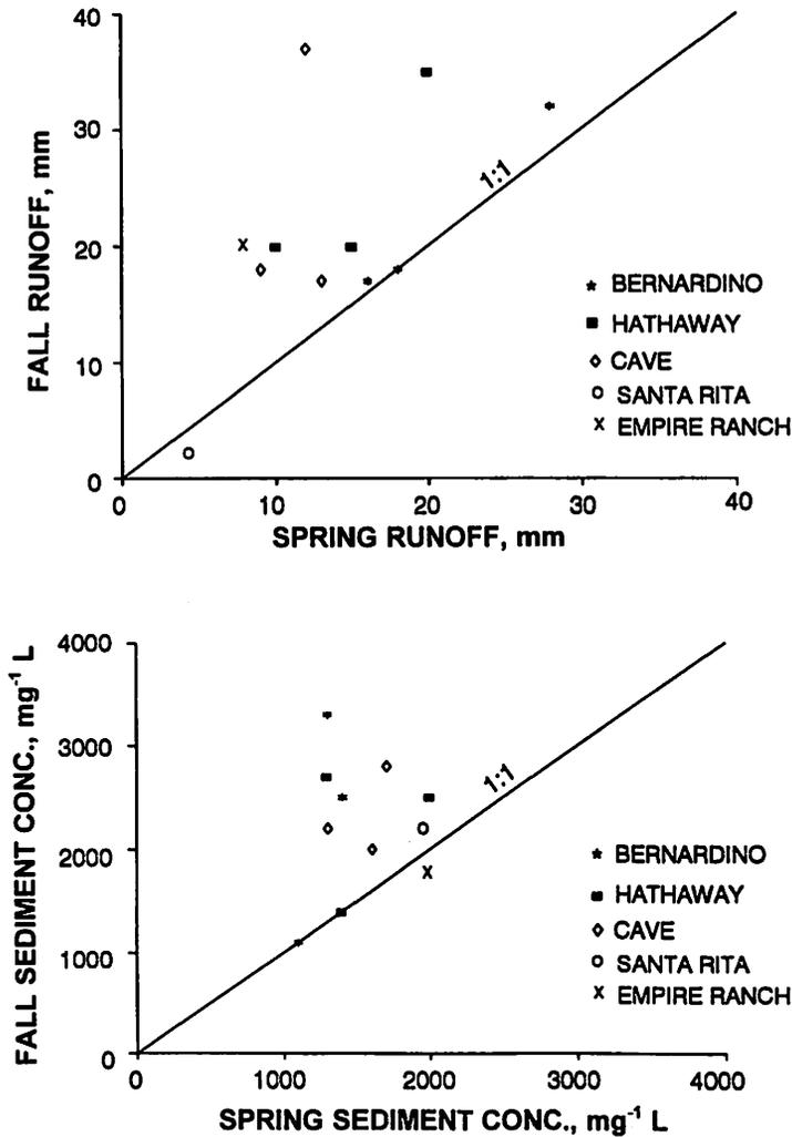
Fig. 5-3. Relation between spring and fall runoff volumes and average sediment concentrations on nonvegetated (bare, clipped, and burned) plots for all study sites.
