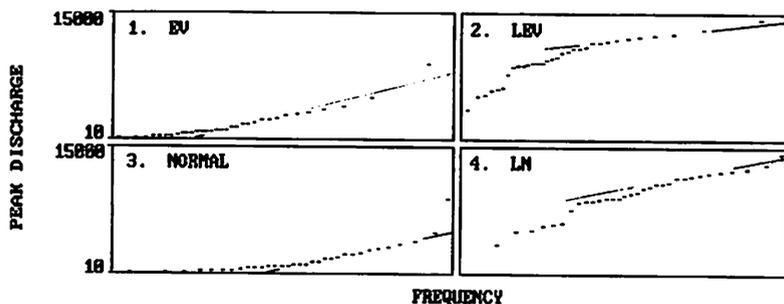
Fig. 1. Annual maximum floods plotted according to Cunnane's formula on N, LN, EV, and LEV graph papers.
