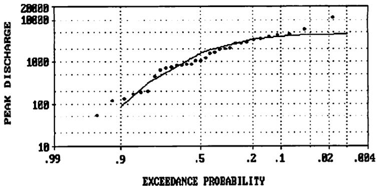
Fig. 2. LP3 math curve does not climb toward four observations between 5,000 and 12,000 cfs.
