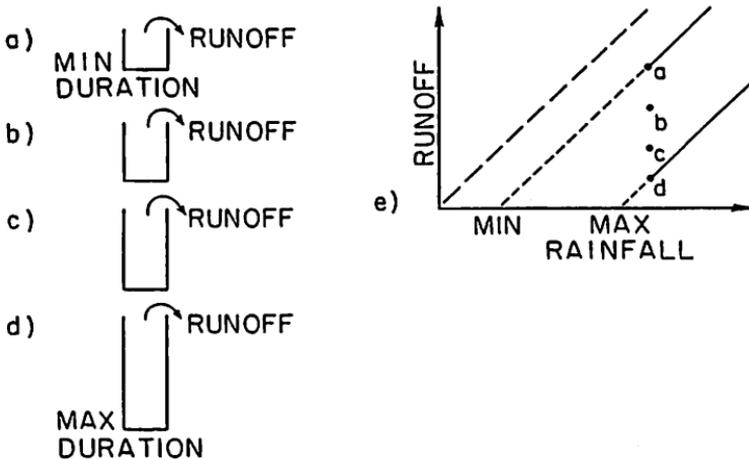
FIG. 8. Effect of Precipitation Duration on "Bucket Model"
