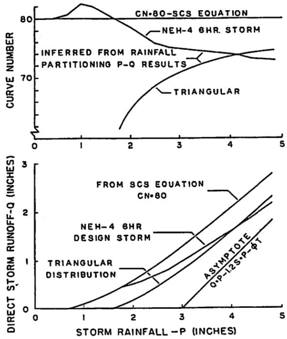
FIG. 10. Comparisons of Runoff and Apparent Curve Number for Six-Hour Storm with CN = 80, by NEH-4 Method and by Rainfall Partitioning for NEH-4 Six-Hour Design Storm and Triangular Distribution of Storm Intensities
