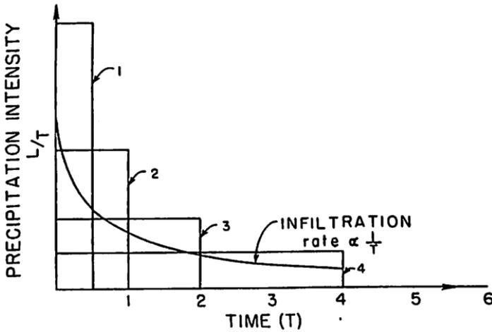
FIG. 7. Schematic Diagram of Four Different Hyetographs
