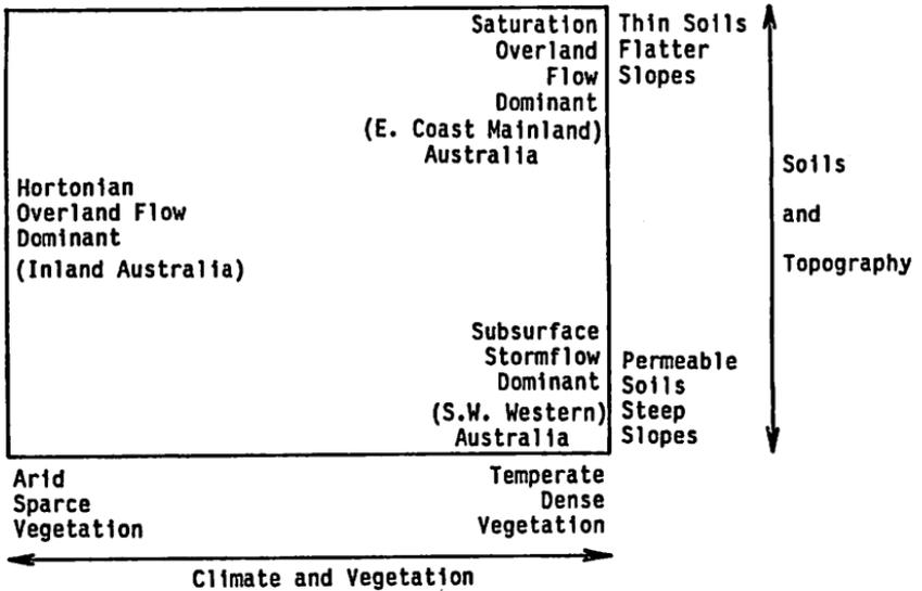
FIG. 11. Proposed Influences of Climate, Soils, Vegetation, and Topography on Runoff-Generating Processes (Adapted from Dunne 1983)
