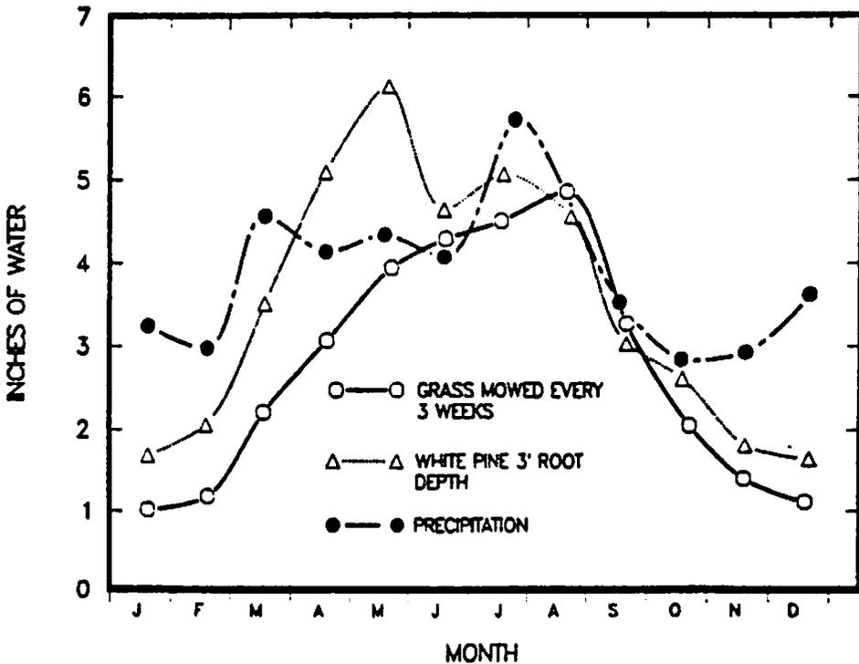
FIGURE 5. Predicted precipitation and evapotranspiration through a soil trench cap at Maxey Flats, Kentucky, 1959-1978, as a function of plant cover and management practice.
