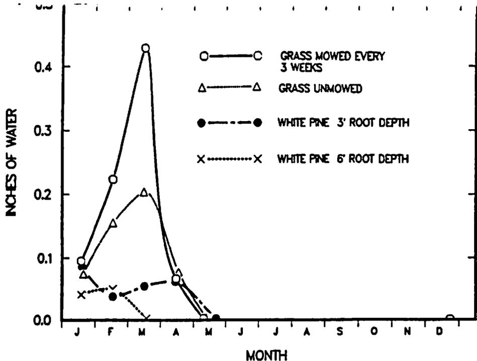
FIGURE 6. Predicted percolation through a 90 cm thick soil trench cap at Maxey Flats, Kentucky, 1959-1978, as a function of plant cover and management practice.
