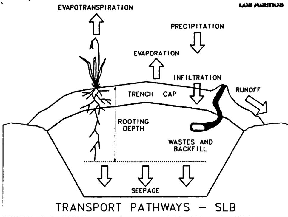
FIGURE 1. Hydrologic processes effecting shallow land burial sites.
