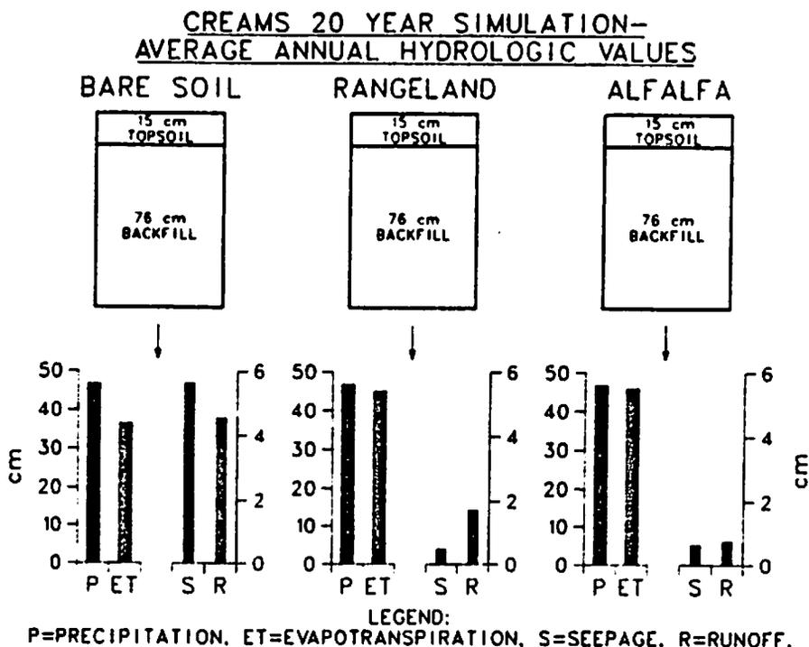
FIGURE 2. Predicted Average annual hydrologic values for a soil over sandy backfill trench cap at Los Alamos, N.M., 1951-1970. (from ref. 22).
