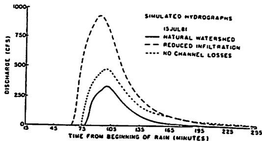
Figure 4. Simulated hydrographs for three land uses for watershed 63011.
