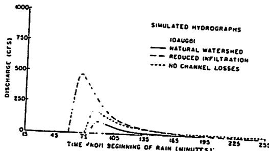
Figure 6. Simulated hydrographs for three land uses for watershed 63011.
