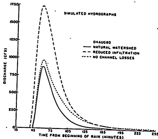
Figure 5. Simulated hydrographs for three land uses for watershed 63011.
