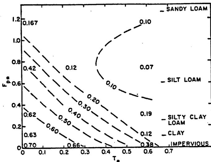
Figure 4a. Kolmogorov-Smirnov  $D_*$  as a function of  $F_{p*}$  and  $T_*$  (constant intensity).
