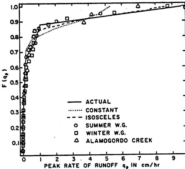
Figure 3c. Empirical distribution functions of peak discharge.  $F_{p*} = 0.290$ ,  $T_* = 0.585$  (Case No. 9).
