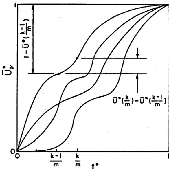
Figure 1. Definition sketch of dimensionless rainfall process  $\bar{U}^*(t_*)$
