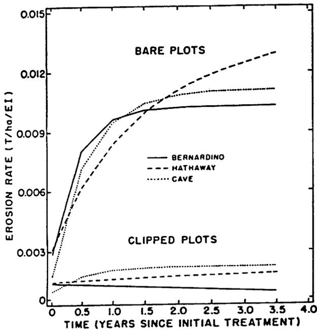
Figure 1. Computer fitted function of actual erosion and time data for the 2 replication average for spring and fall runs with time zero equal to spring 1981 for the Walnut Gulch bare and clipped plots.
