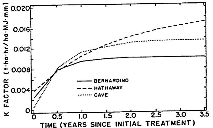
Figure 6. Computer fitted function of USLE K factor change with time for the Walnut Gulch bare plots. Time zero equals spring 1981 and C was assumed 1 for the bare surface condition.
