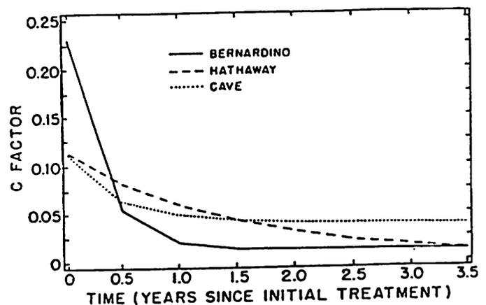
Figure 9. Computer fitted function of USLE C factor change with time where time zero equals spring 1981 for the Walnut Gulch natural plots. The C factor was calculated using the simulator derived K value from the bare plots whose C value was assumed to be 1.
