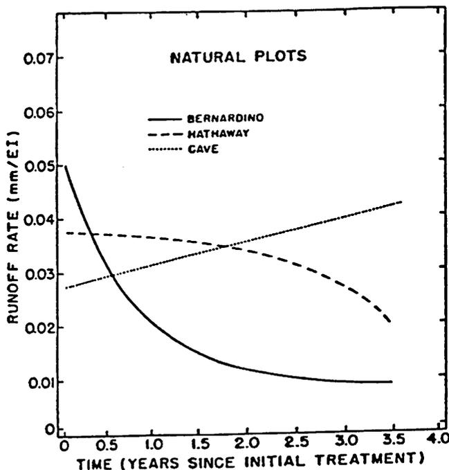
Figure 5. Computer fitted function of actual runoff rate and time data for the 2 replication average for spring and fall runs with time zero equal to spring 1981 for the Walnut Gulch natural plots.
