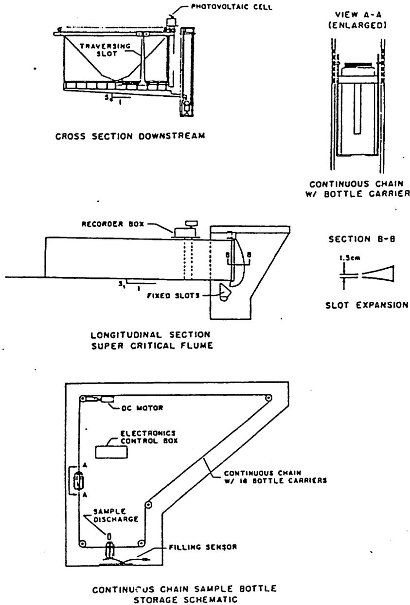
Fig. 2. Schematic diagram of slot sampler mechanism.
