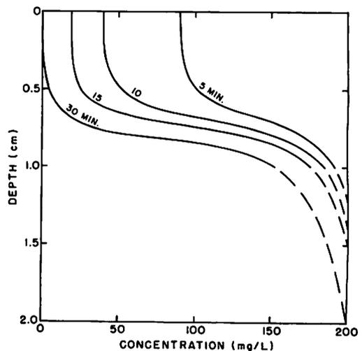
Fig. 6—Average concentration profile (slope = 0; infiltration = 0.434 cm/h).
