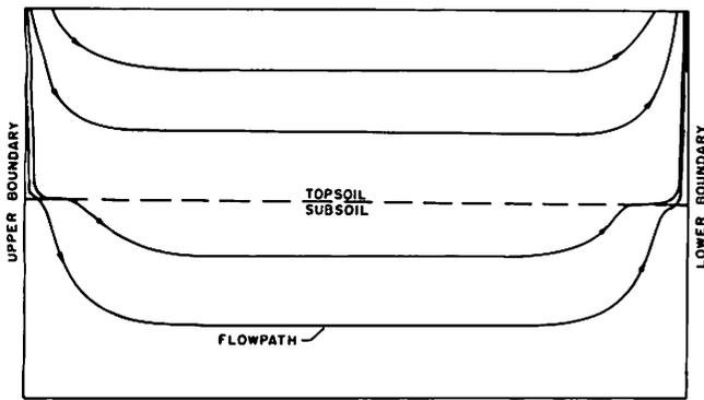
Fig. 7—Predicted flow paths through a two-layer porous media system having a 3% slope and no infiltration.
