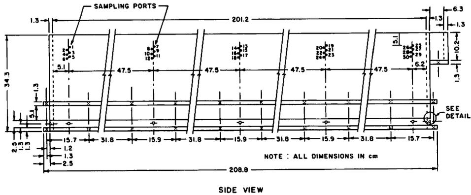
Fig. 1a—Side view of soil flume showing location and numbering of sampling points.
