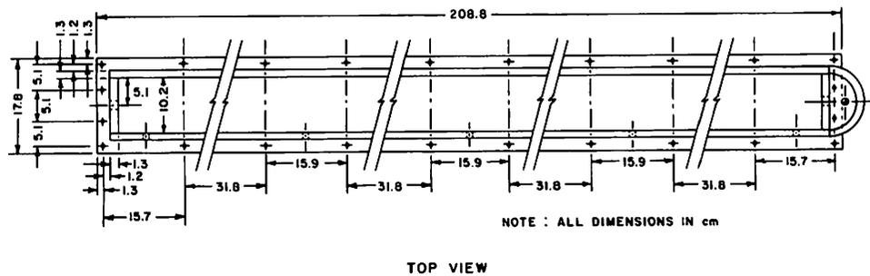
Fig. 1b—Top view of soil flume.
