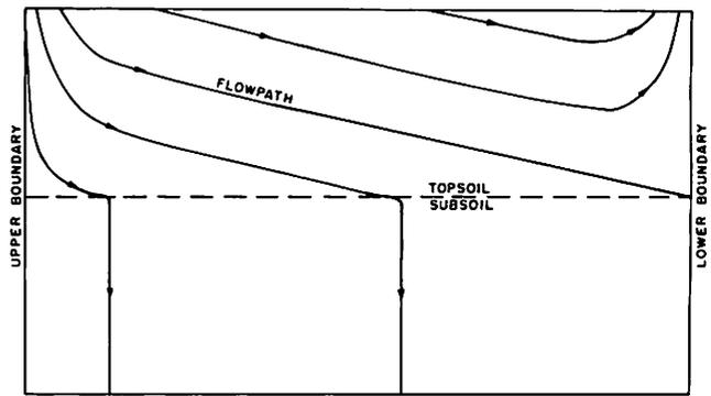
Fig. 9—Predicted flow paths through a two-layer porous media system having a 3% slope and a positive infiltration rate.
