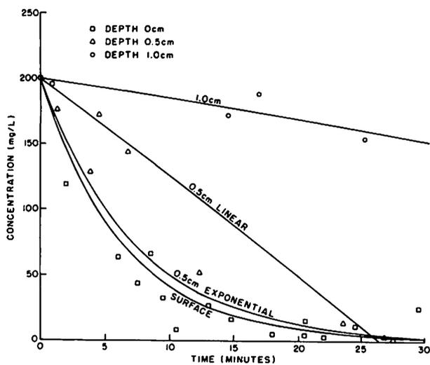
Fig. 4b—Concentration vs. time (infiltration = 0.434 cm/h).
