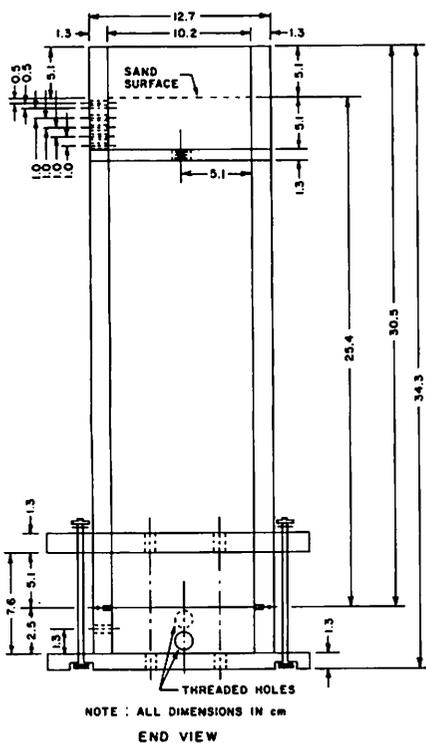
Fig. 1c—End view of soil flume.
