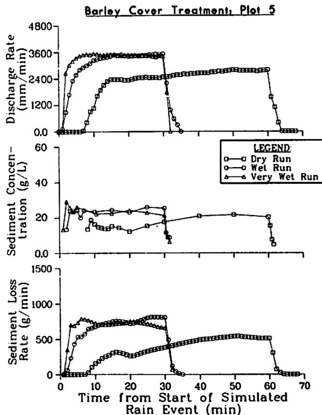
Fig. 5—Hydrograph, sediment concentration, and sedigraph data from plot 5 with barley cover.
