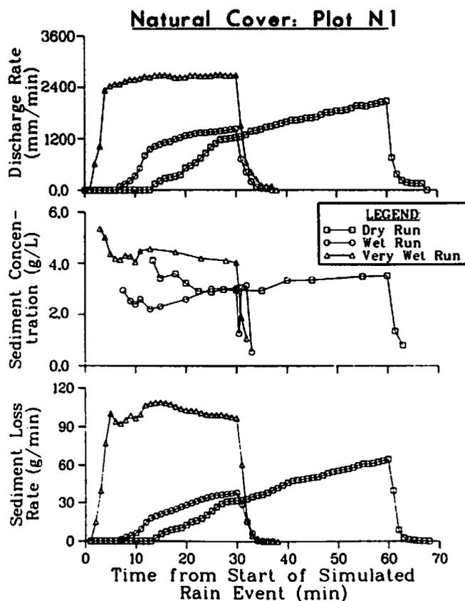
Fig. 1—Hydrograph, sediment concentration, and sedigraph data from natural cover plot N1.
