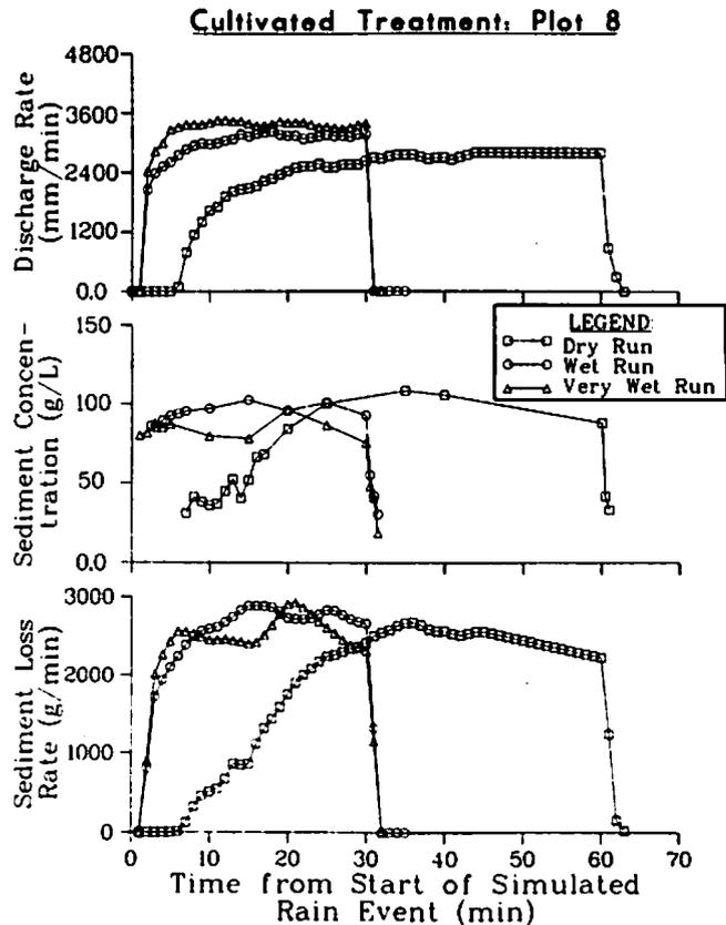
Fig. 3—Hydrograph, sediment concentration, and sedigraph data from plot 8 with cultivated treatment.
