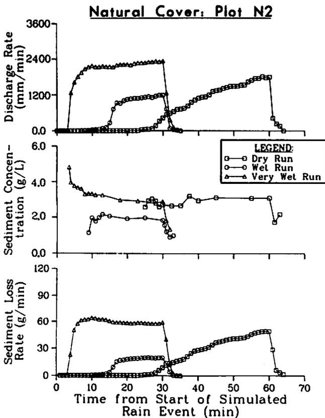
Fig. 2—Hydrograph, sediment concentration, and sedigraph data from natural cover plot N2.
