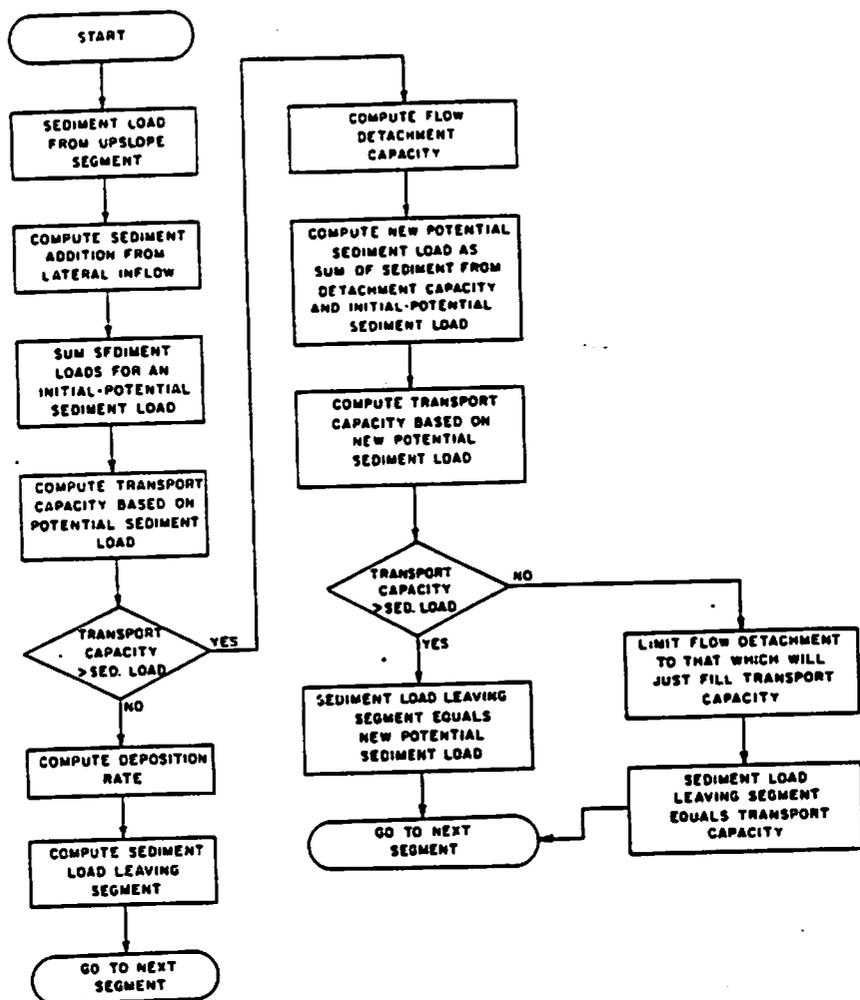
FIG. 2 Flow chart for detachment-transport-deposition computations within a segment of an overland flow or channel element.
