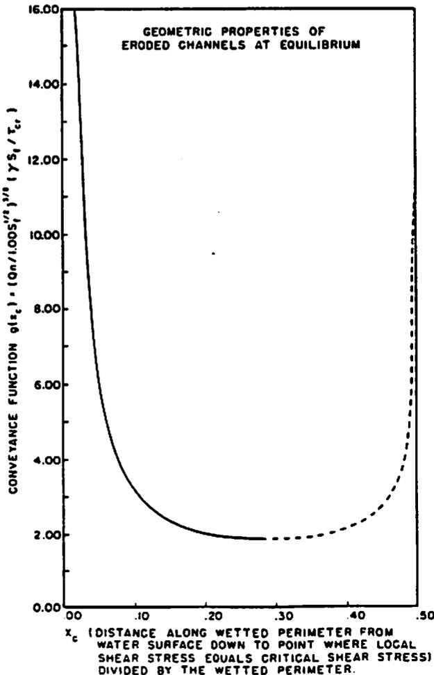
FIG. 4 Function  $g(x_c)$  for an eroding channel at equilibrium.
