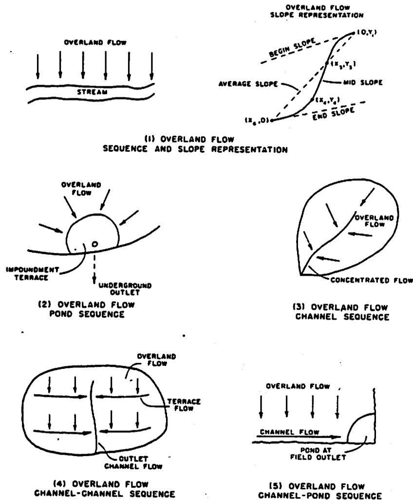
FIG. 1 Schematic representation of typical field systems in the field-scale erosion/sediment yield model.
