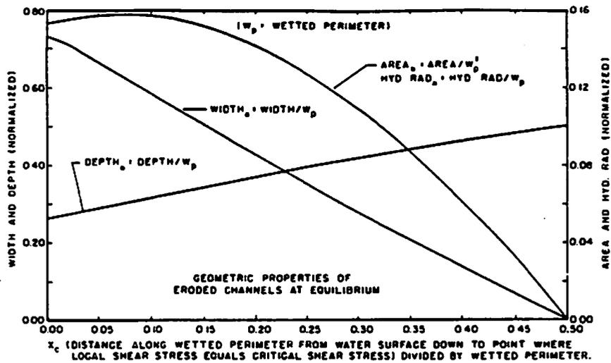
FIG. 3 Geometric properties of an eroding channel at equilibrium.
