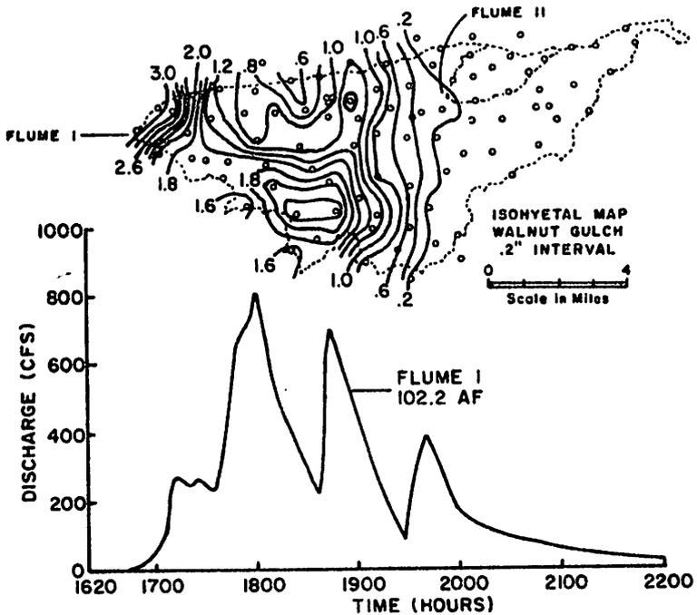
FIG. 7.—Storm of August 25, 1968 Was Concentrated in Lower Portion of Watershed; Multip peaked Hydrograph Resulted from Runoff in Various Tributaries and from Longer Duration Hyetograph with Several Periods of Precipitation Excess
