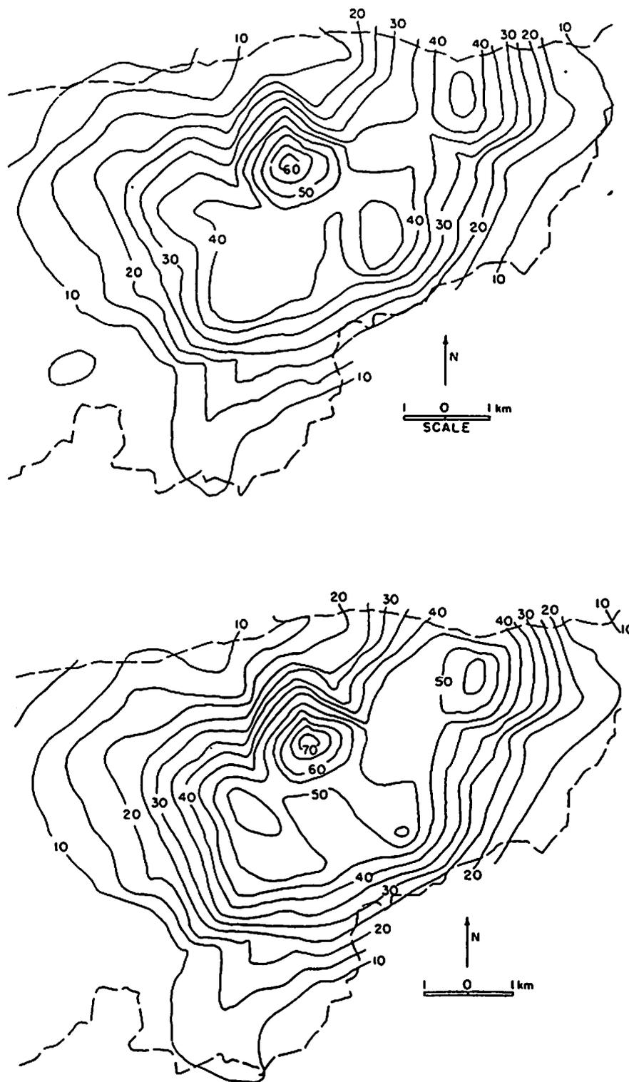
Fig. 6. Maximum 30-min (top) and 60-min (bottom) rainfall (in millimeters) for Walnut Gulch W-6 subwatershed on September 10, 1967, prepared using data from the 1957 network only.
