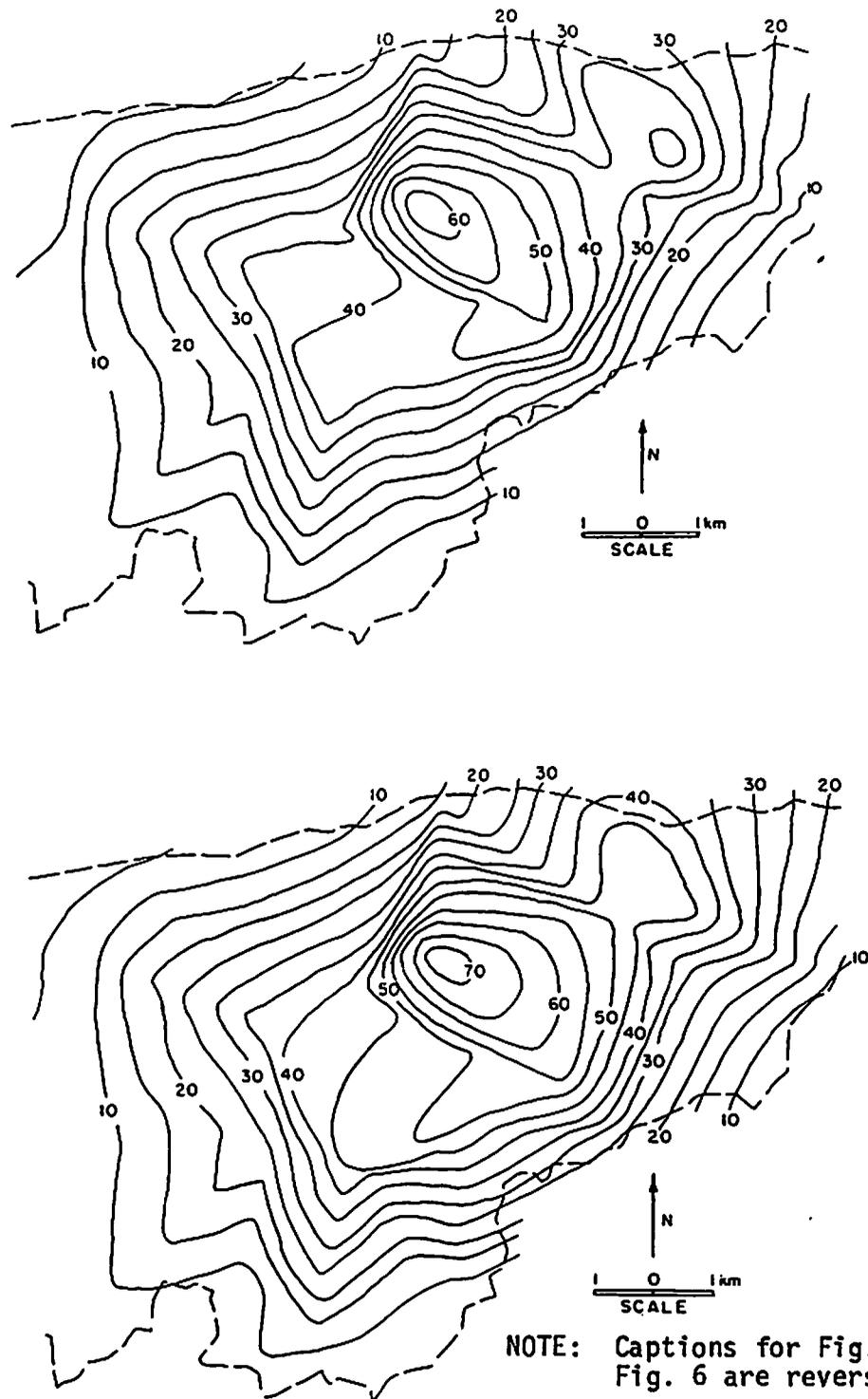
Fig. 5. Maximum 30-min (top) and 60-min (bottom) rainfall (in millimeters) for Walnut Gulch W-6 subwatershed on September 10, 1967, disregarding rain gage 52.
