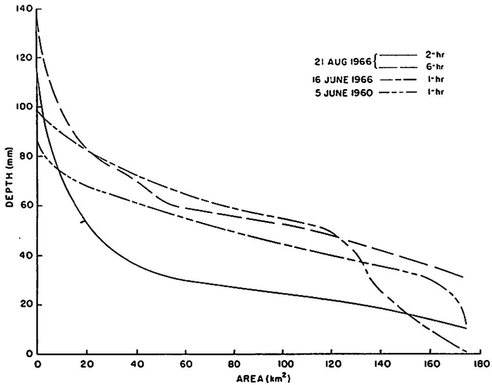
Fig. 10. Depth-area rainfall curves for three storms on Alamogordo Creek.
