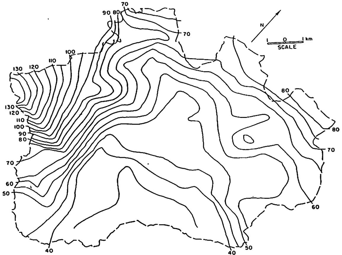
Fig. 8. Maximum 6-hour rainfall (in millimeters), August 21, 1966, Alamogordo Creek.
