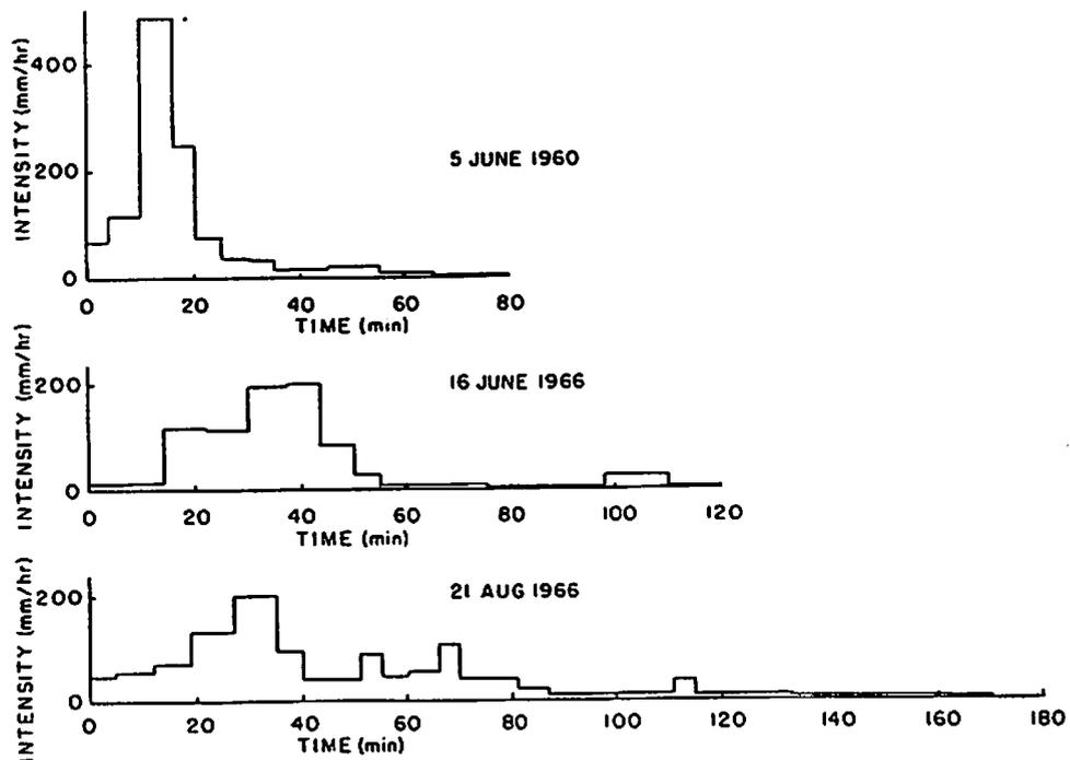
Fig. 9. Rainfall intensity with time for gages recording maximum rainfall for three selected storms on Alamogordo Creek.
