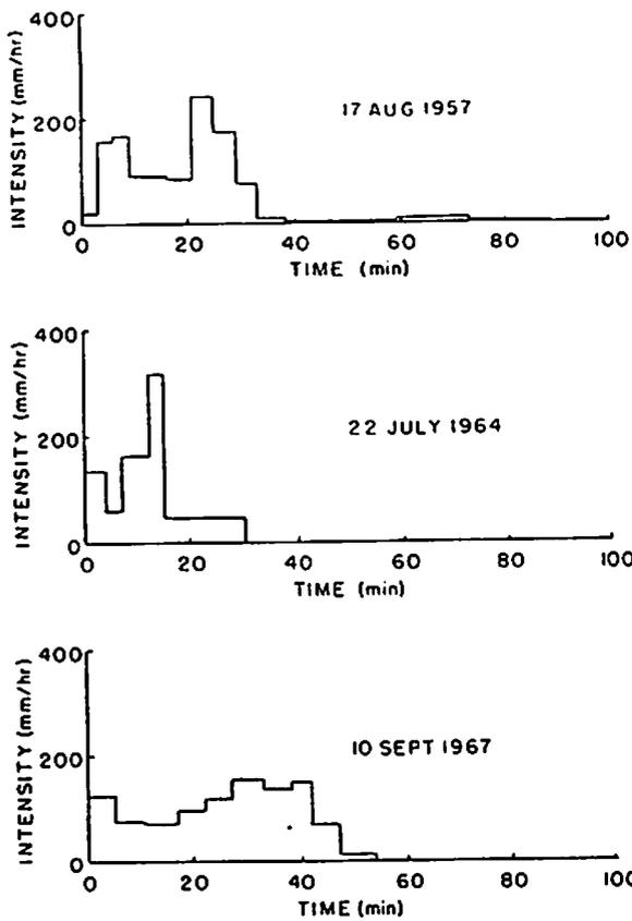
Fig. 3. Rainfall intensity with time for gages recording maximum rainfall for three selected storms on Walnut Gulch.
