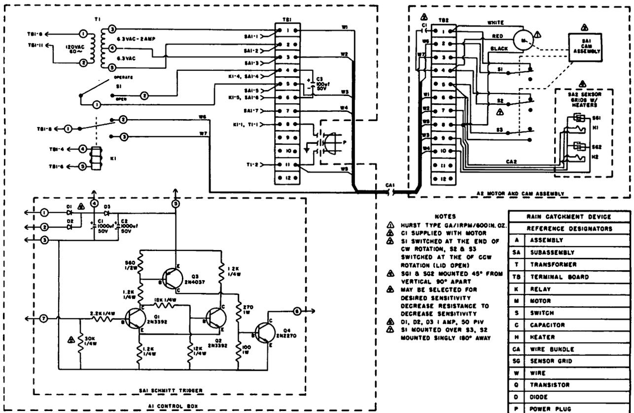
Figure 2.--Schematic diagram of circuitry for lower and upper control boxes, including the Schmitt trigger.
