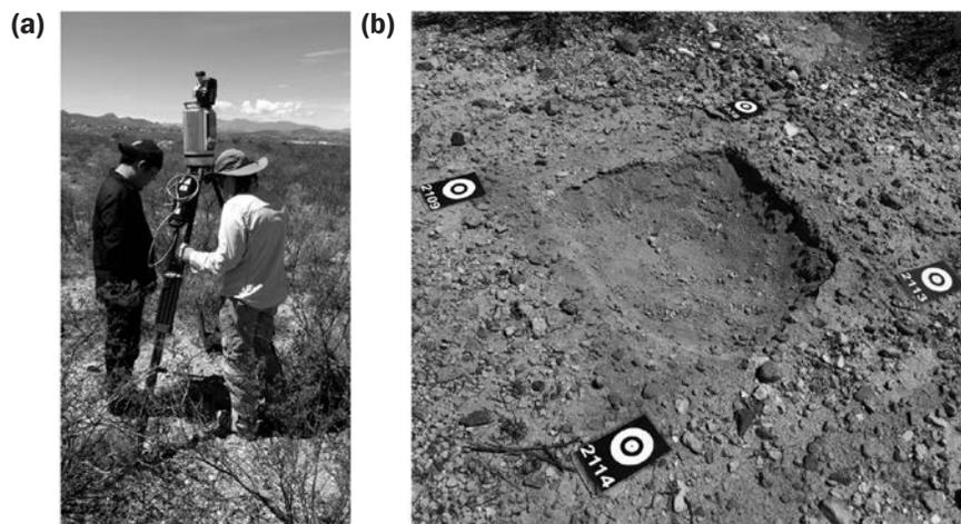
out any noise along the edges. The change in volume between scan sets (i.e., loose rock surface, bare surface, and excavated surface) was determined using the Surfer Grid Volume tool.
