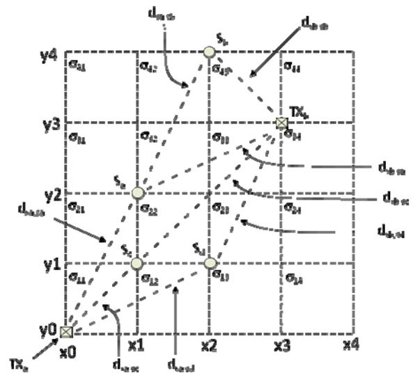
Figure 10. Illustration of how transmitters (TX) and sensors (S) can be used to construct the conductivity ( $\sigma$ ) on a square grid assuming a known conductivity and distance between transmitters and sensors.
