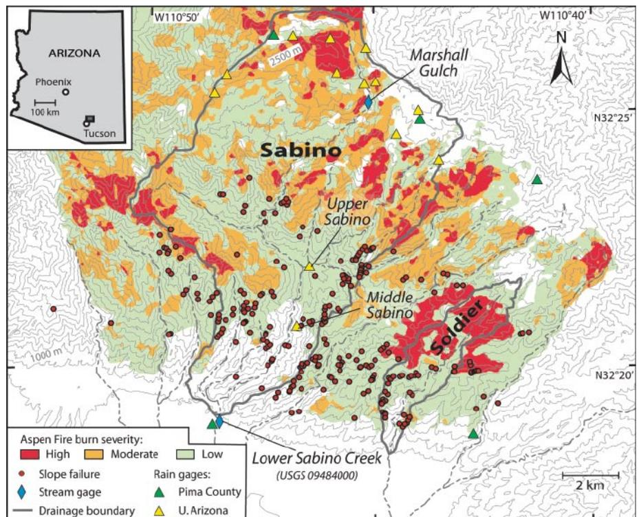
Fig. 1. Map of hillslope failures, rainfall gages, and stream gages within the Santa Catalina Mountains north of Tucson, Ariz. The elevation contour interval is 100 meters. Locations of hillslope failures were mapped with helicopter-based and ground-based reconnaissance.
