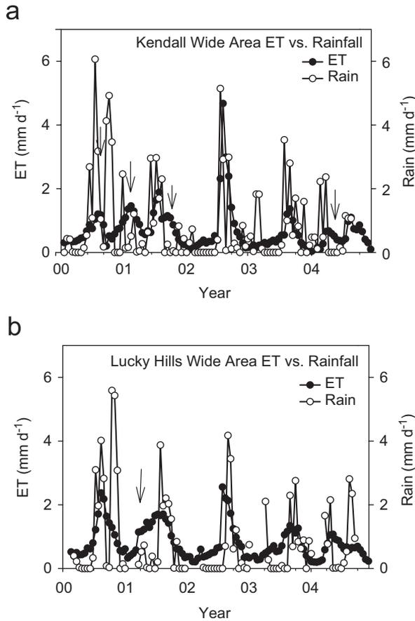
Fig. 4. Time course of projected ET and  $P$  at Kendall (a) and Lucky Hills (b) wide area sites. Arrows show extended periods when ET exceeded  $P$ .
