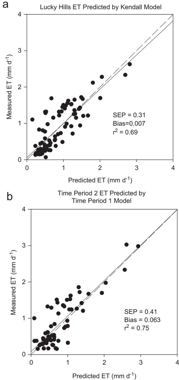
Fig. 3. Cross validation plots, showing measured ET at the Lucky Hills site plotted against predicted ET based on a regression equation developed from Kendall data (a); and measured ET for the second half of the study (period 2) plotted against predicted ET based on a regression equation developed from period 1 data (b). The solid lines in each plot show regression lines of best fit while the dashed lines are 1:1 lines.
