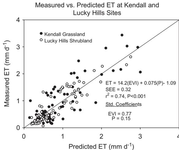
Fig. 2. Equation of best fit for predicting measured ET from EVI and *P* at Kendall and Lucky Hills tower sites in the Upper San Pedro River Basin.
