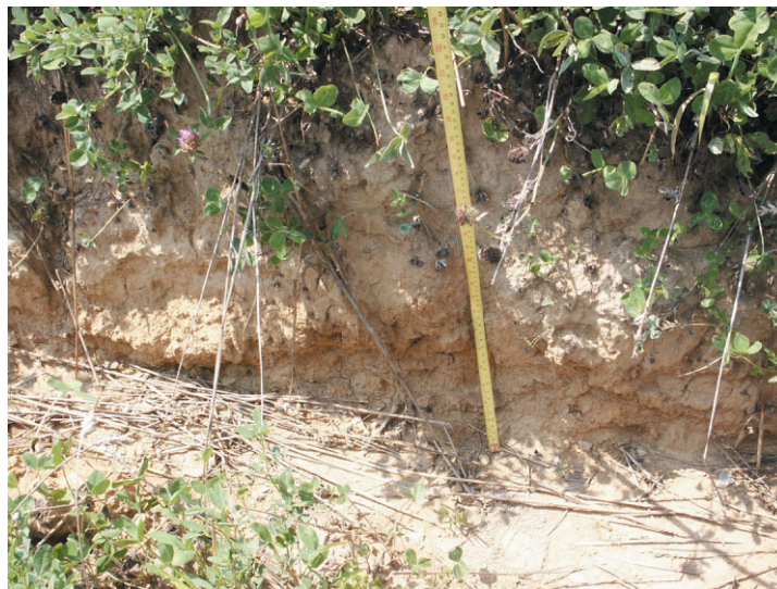
Figure 6. Deeply incised area on the channel element at the end of the experimental period. This figure is available in colour online at www.interscience.wiley.com/journal/espl
