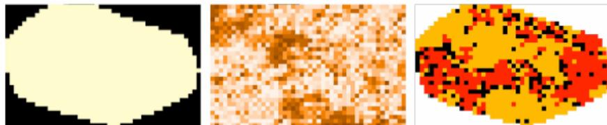
Figure 1. The LCMF process. (left) The modification area; (middle) the multifractal surface generated from the 2D midpoint displacement algorithm; and (right) the final randomly distributed, patchy land cover surface for 3 land cover classes.
