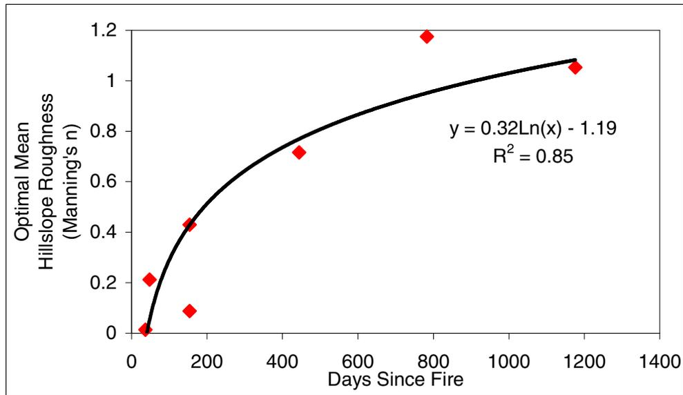
**Figure 4 – Optimal Hillslope Roughness for Events that Occurred after the Cerro Grande Fire at Starmer Canyon Plotted vs Time**
