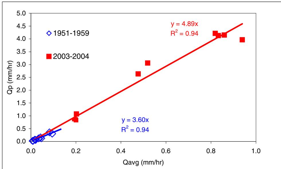
**Figure 2 – Peak Discharge plotted against Average Discharge for Before and After the Marshall Gulch Fire**
