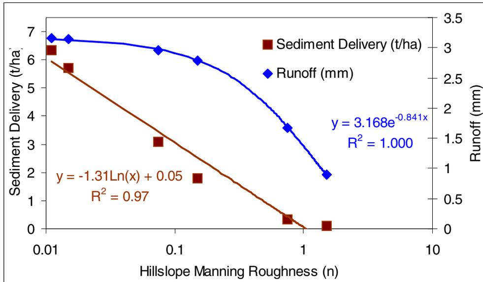
**Figure 8 – Hillslope Sediment Delivery and Runoff Volume Plotted vs hillslope roughness values**
