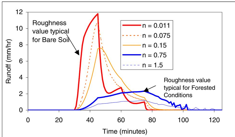
**Figure 6 – Hillslope Runoff Plotted vs time for Different Hillslope Roughness Values**
