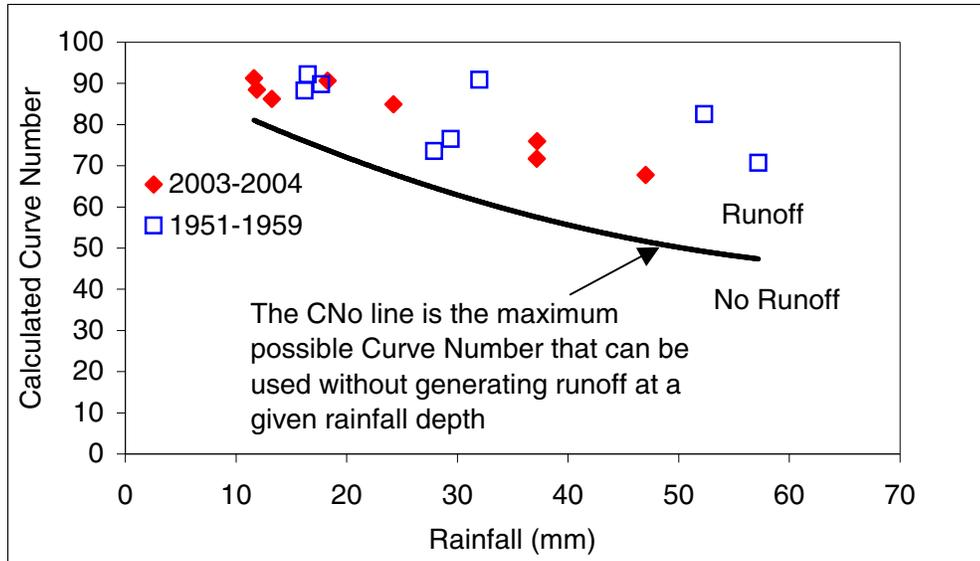
**Figure 1 – Calculation of Curve Numbers before and After the Marshall Gulch Fire**
