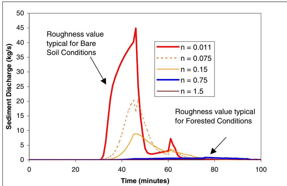
**Figure 7 – Hillslope Sediment Discharge Plotted vs Time for Different Hillslope Roughness Values**
