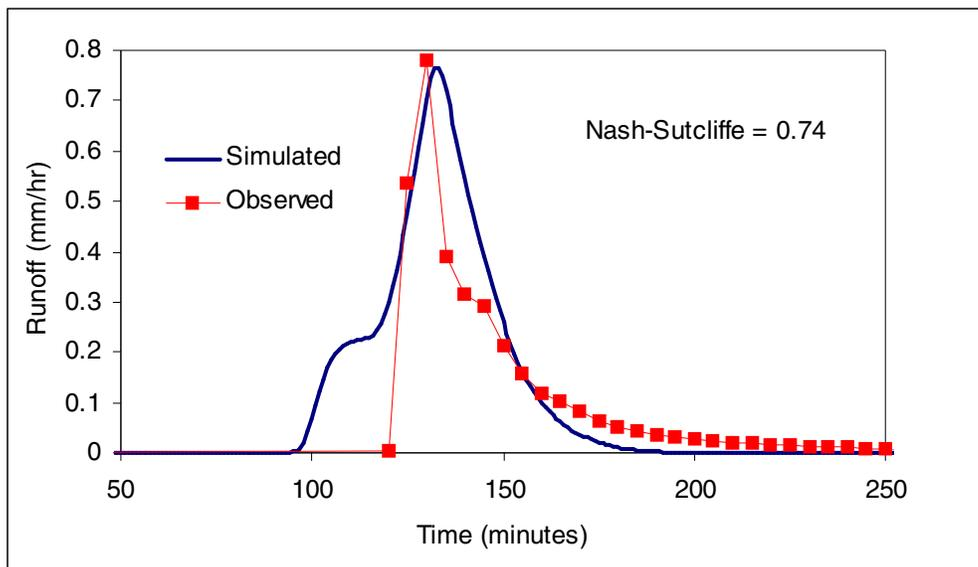
**Figure 3 – Comparison of Observed and Simulated Hydrograph for the Poorest fit Hydrograph Used in the Analysis at Starmer**
