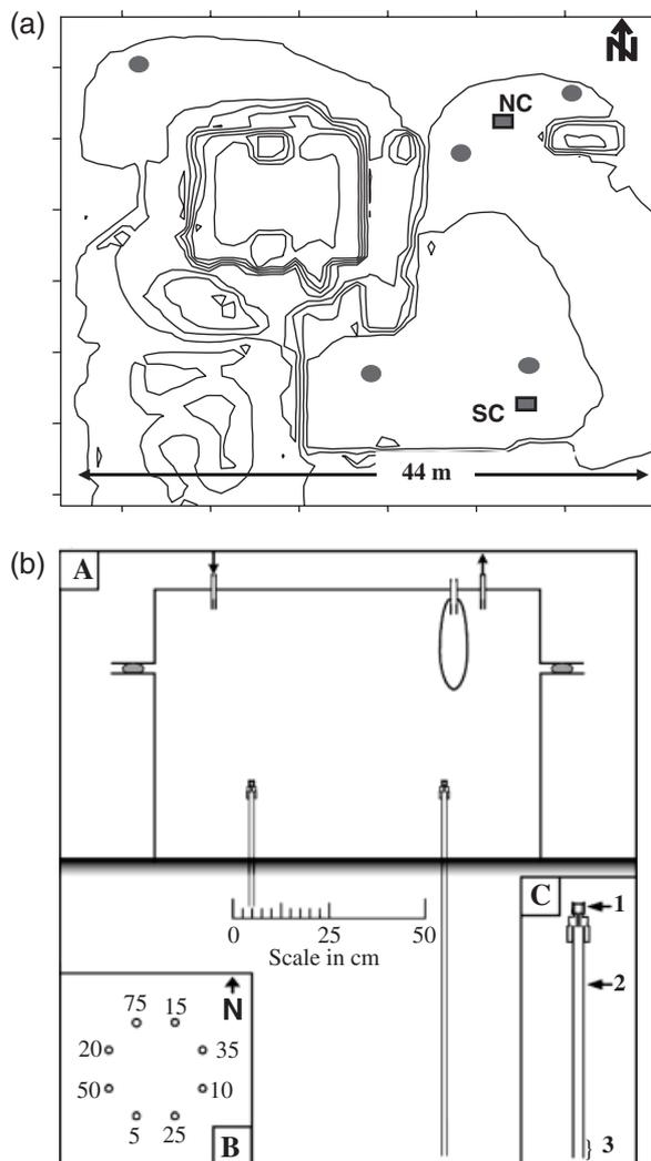
**Fig. 1** (a) Rainforest contour (thin lines) map with soil moisture probe and chamber locations and (b) diagram of soil chamber and probe sampling setup. (a) Chamber and probes in cross-section are shown; (b) contains a map outlining probe locations (borders represent the large chamber dimensions); and (c) a detailed drawing of probe design.
