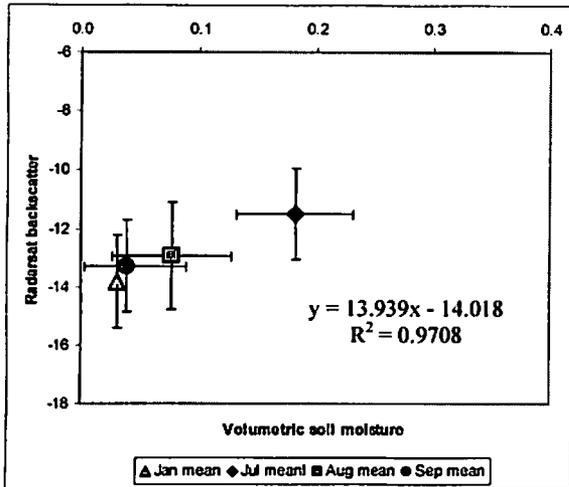
Figure 2. Relationship between mean volumetric soil moisture and mean Radarsat backscatter at the watershed scale. Backscatter and soil moisture were averaged by date for the 44 field sites. Soil moisture for the January image was not measured, but assumed to be 3% at all sites.
