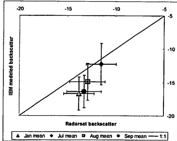
Figure 3. Observed radar backscatter versus modeled radar backscatter for 35 x 35 m<sup>2</sup> areas in 2003. Each point is an average of 44 sites.
