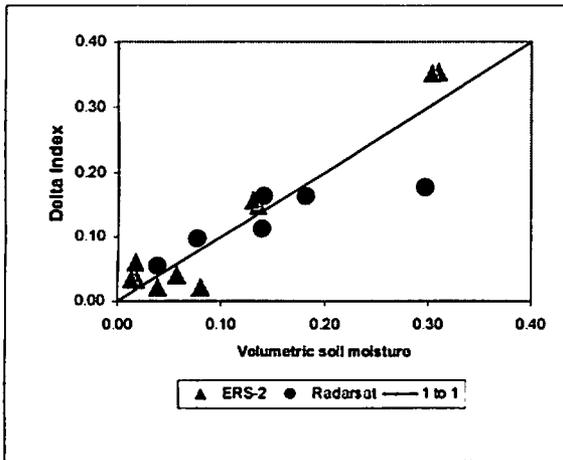
Figure 5. Delta index and volumetric soil moisture for field conditions sensed by both ERS and Radarsat satellites.
