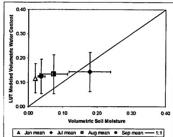
Figure 4. Predicted volumetric water content obtained through IEM generated LUT versus field volumetric water content on four dates in 2003. Soil moisture for the January period was not measured, but assumed to be 3%.
