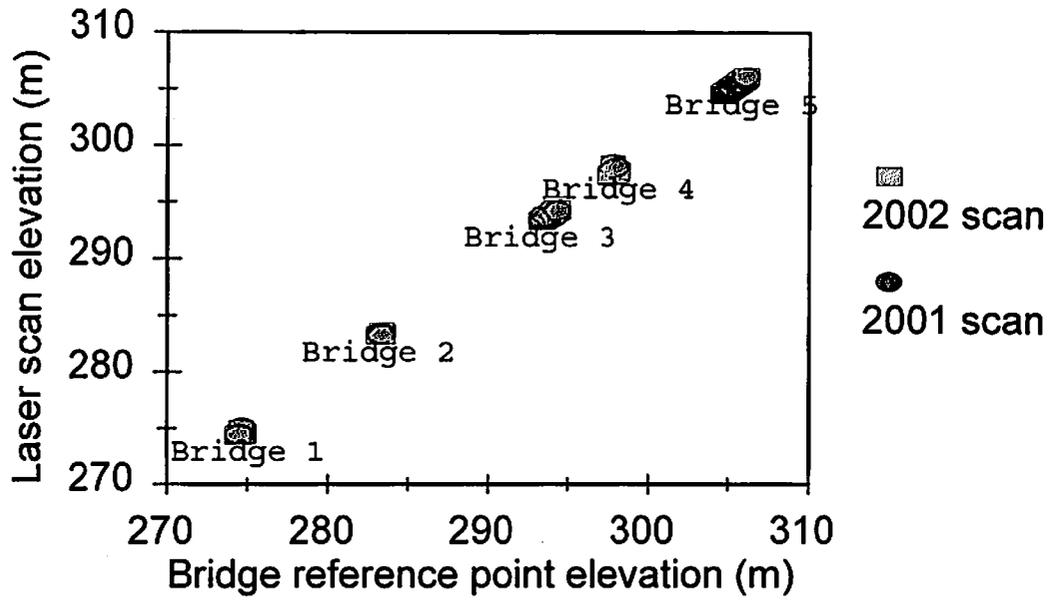
Figure 2. Correspondence of bridge surface elevations obtained via RTK-GPS survey on the ground versus elevations for the same surfaces determined by 2001 and 2002 LIDAR.
