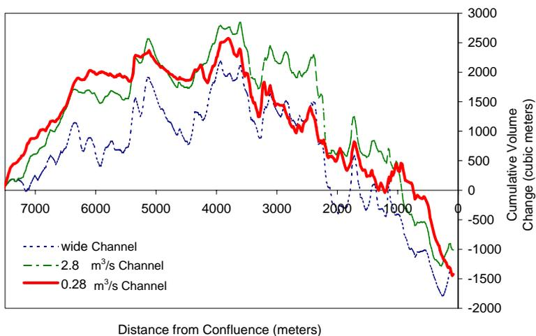
Fig. 6. Comparison of different conceptual representation on scour and deposition.
