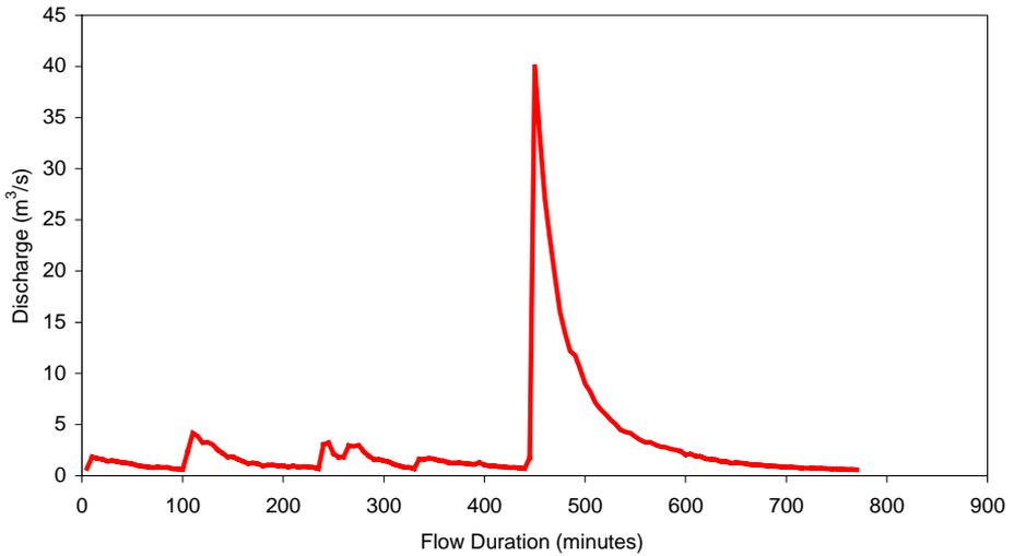
Fig. 1. The observed hydrograph in Pueblo Canyon for the period from August 2000 to July 2001. Events with peaks less than  $1.7 \text{ m}^3/\text{s}$ , and periods of no flow have been removed to create one continuous hydrograph for input into HEC6T.
