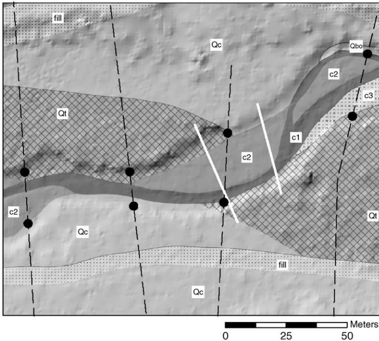
Fig. 7. The left and right bank stations in the HEC6T simulation correspond to the limits of the channel geomorphic units. The C1 and C2 units shown on the map correspond to the channel units mapped by *Reneau et al. (1998)*. The left and right bank stations on a cross-section, which are selected based on the limits of a 2.8 m<sup>3</sup>/s flow, are given by the ● symbol.
