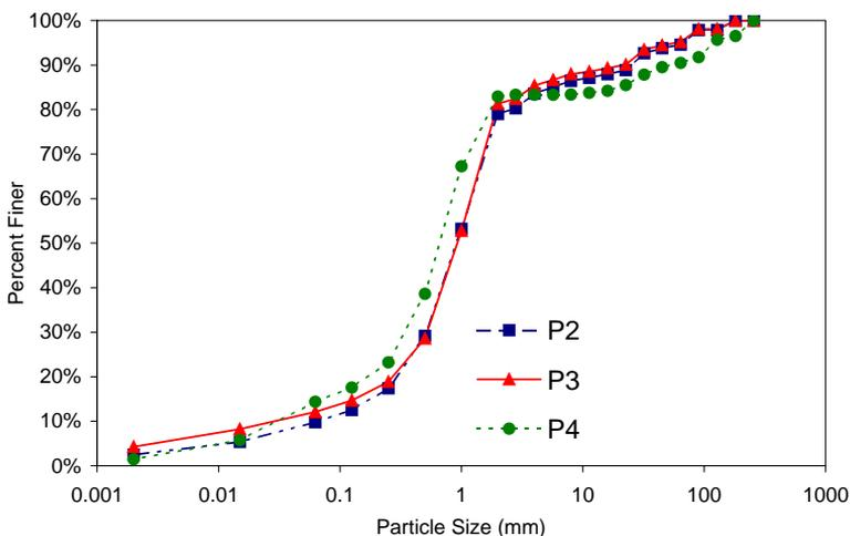
Fig. 5. Percent finer curves for three reaches based on the data of Reneau et al. (1998). The cross-sections where these particle sizes apply are listed next to the reach number.
