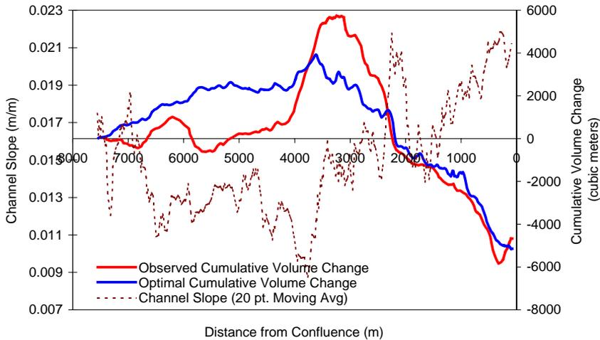
Fig. 9. Comparison of model cumulative scour, observed cumulative scour and channel slope.
