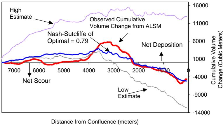
Fig. 8. Comparison of model cumulative scour for a high, low and optimal estimate in comparison with observed cumulative scour.
