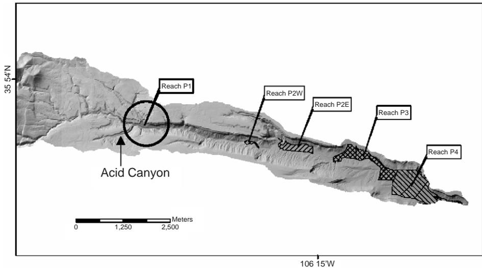
Fig. 2. Diagram of Pueblo Canyon. HEC6T was used to model scour and deposition in Pueblo Canyon from just above Acid Canyon to the confluence with Los Alamos Canyon. The reaches described in the Pueblo Canyon Reach Report (Reneau et al., 1998) are shown on this figure.
