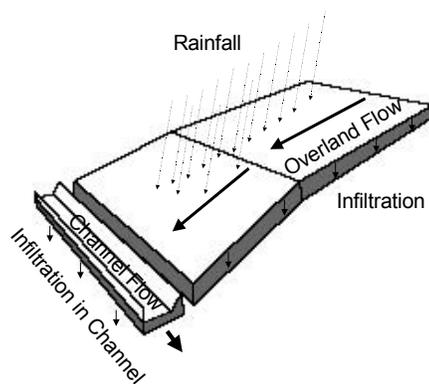
Figure 2. A schematic representation of the geometric representation of hillslopes and channels in the KINEROS2 model as well as the runoff processes simulated in the model.
