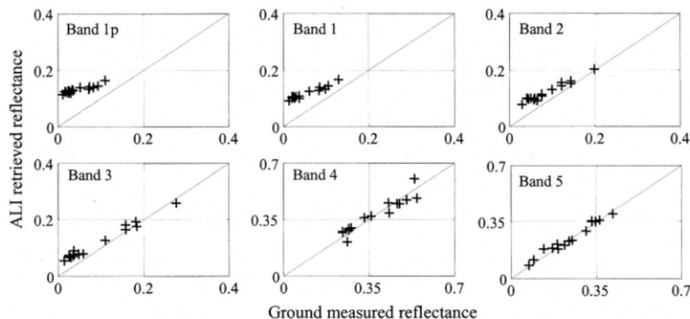
Fig. 2. Reflectance retrieved from ALI with no atmospheric correction [(3)] compared to ground-measured reflectance for 15 targets at MAC and WGEW on six dates.
