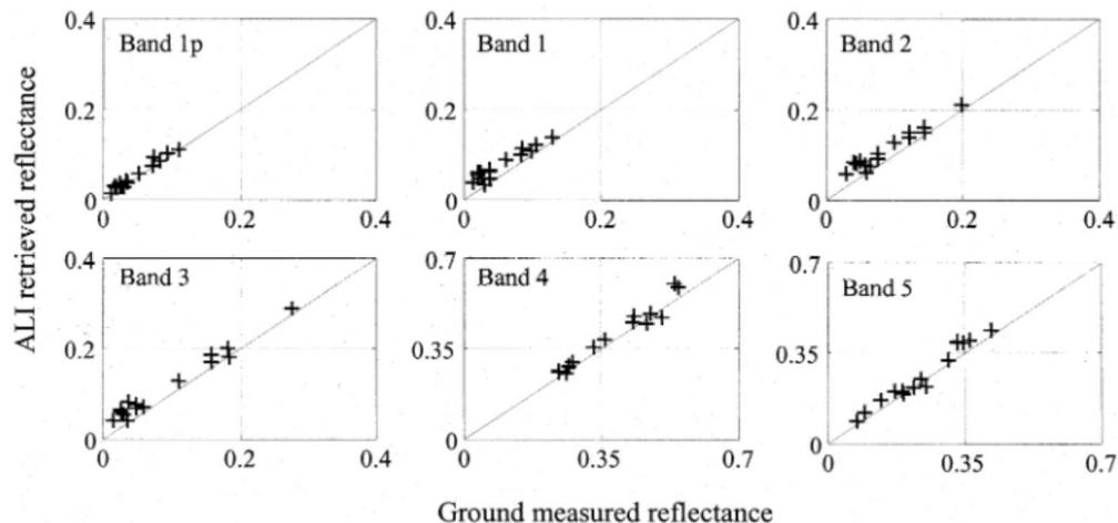
Fig. 1. Reflectance retrieved from ALI using the REL approach [(1)] compared to ground-measured reflectance for 15 targets at MAC and WGEW on six dates (from Table III). To conserve space, results from only six of nine ALI bands are presented, where band 4 represents results for the NIR spectrum, and band 5 represents results for the SWIR spectrum.
