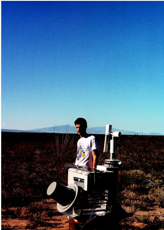
Fig. 4. The CIMEL sunphotometer for measuring aerosol optical depth, at the USDA-ARS Walnut Gulch Experimental Watershed, Tombstone, AZ.
