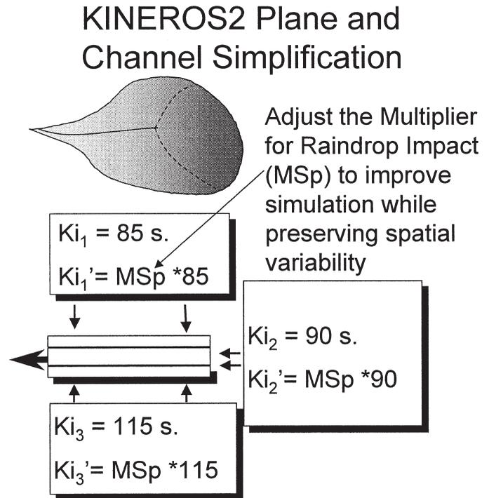
Figure 3. Example of the Use of Multipliers for Parameter Estimation.
