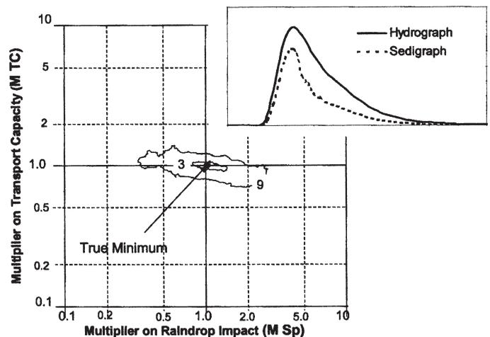
Figure 6. An Error Response Surface for an Identifiable Parameter Case. Contour values are Total Sum of Squared Residuals (TSSR), which have been normalized to the mean of the error response surface.
