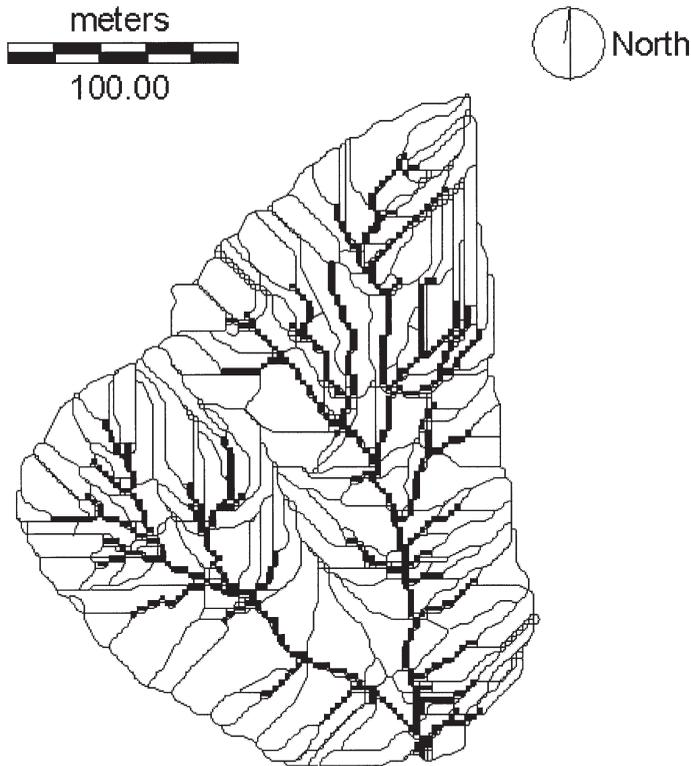
Figure 2. Partitioning of the Lucky Hills Watershed Into 312 Different Plane and Channel Elements for Use in the KINEROS2 Hydrologic Model. The partitioning was done using the TOPAZ DEM Processing Program (Garbrecht and Campbell, 1997), and reflects the channel complexity identified in the field.
