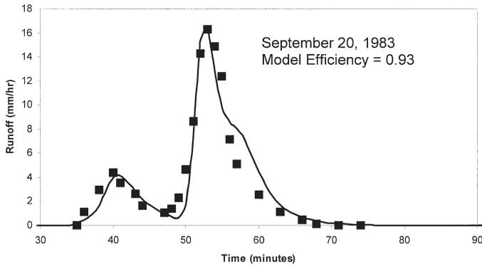
Figure 8. The Worst Hydrograph Used in Simulation. This shows the result of parameter identification for hydrologic variables ( $K_s$ ,  $CVK_s$ , and Manning's  $n$ ).
