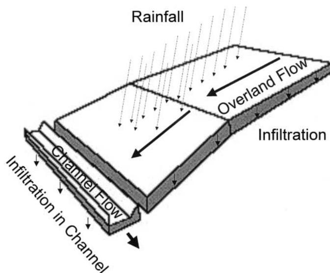
Figure 1. Plane and Channel Representation. Hillslopes in KINEROS2 are represented as a series of cascading planes.
