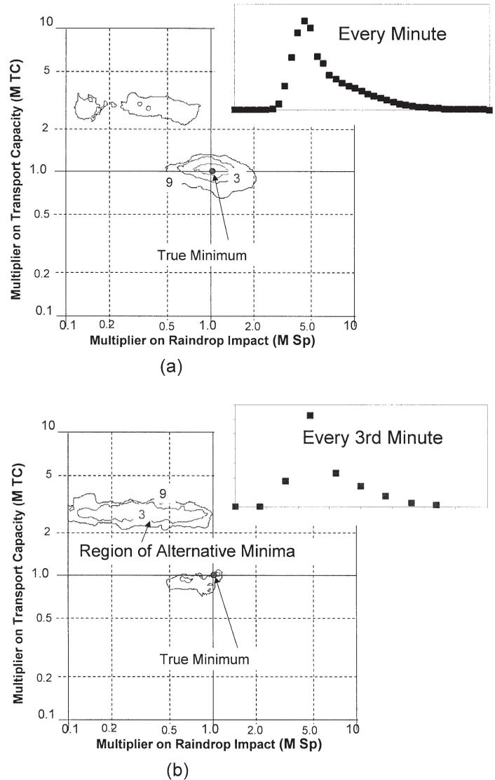
Figure 7. Error Response Surface for a Large Event Comparing the Effect of Sampling Frequency on Parameter Identification. (a) Sedigraph data at one-minute intervals. (b) Sedigraph data at three-minute intervals. Contour values are in TSSR.
