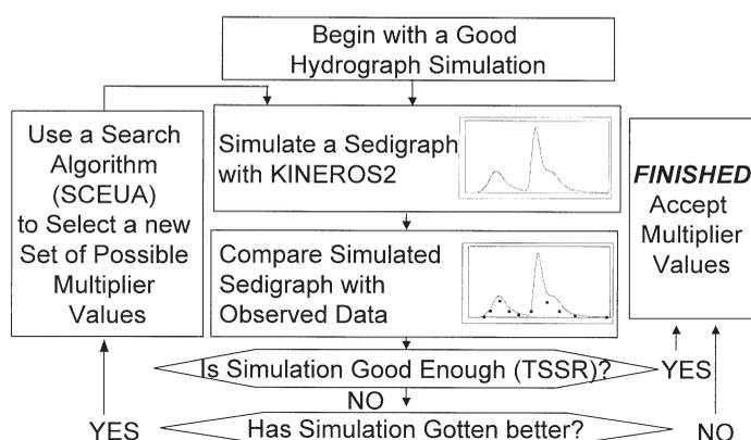
Figure 4. The Method for Parameter Identification Used in This Study. TSSR refers to the total sum of squared residuals. SCEUA refers to the Shuffled Complex Evolution UA (Duan *et al.*, 1992).
