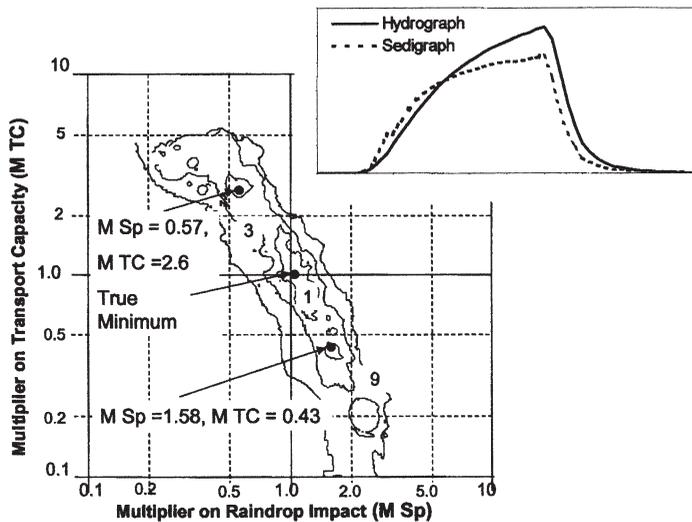
Figure 5. An Error Response Surface for a Poorly Identifiable Parameter Case. Contour values are Total Sum of Squared Residuals (TSSR), which have been normalized to the mean for the error response.
