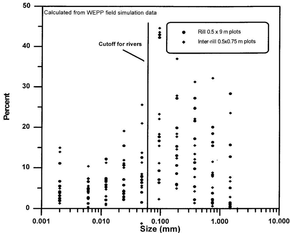
Figure 2. Aggregate sizes in runoff from plots.
