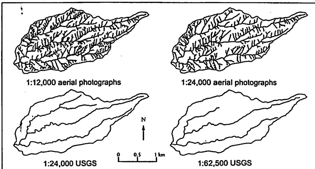
Figure 2. Digitized stream channels within subwatershed 11 on Walnut Gulch. Note how the drainage density decreases with decreasing scale while the underlying structure of the drainage pattern is retained.
