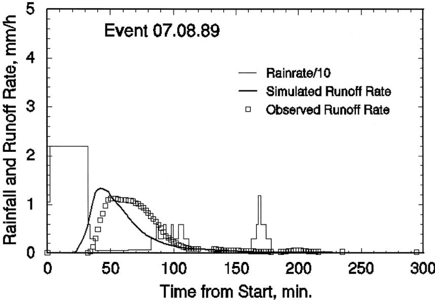
Fig. 9. Measured and simulated runoff for event of 7.8.89.
