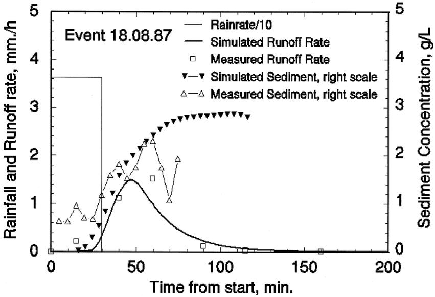
Fig. 3. Calibrated KINEROS2 and measured results for the event of 18.8.87.
