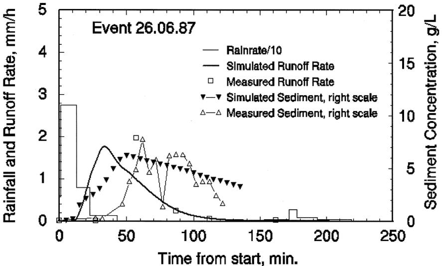
Fig. 4. Calibrated KINEROS2 and measured water and sediment discharges for the event of 26.06.87.
