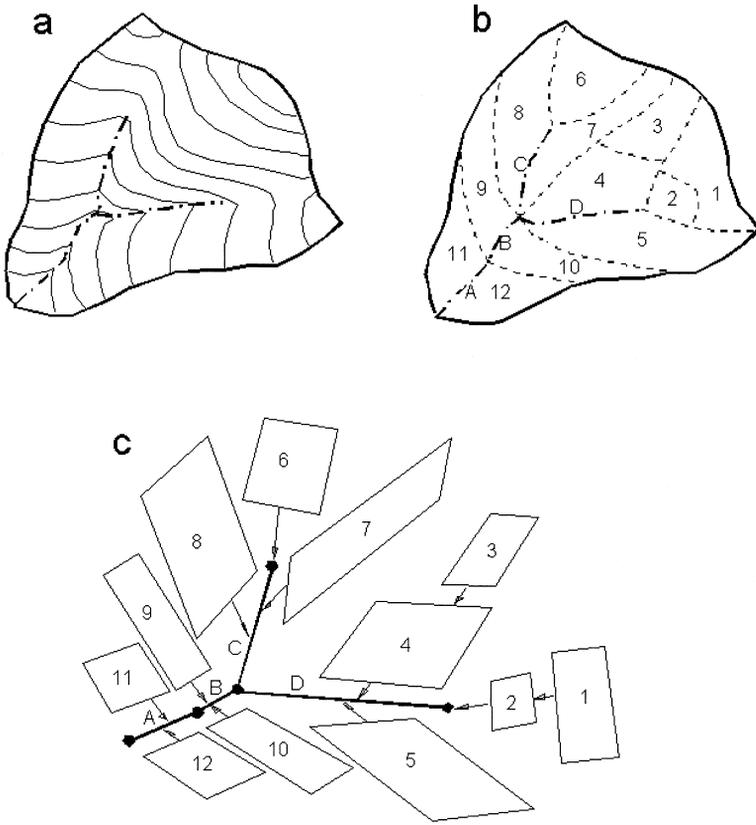
Fig. 1. Schematic illustration of the geometric subdivision of a hypothetical catchment into a network of surfaces and receiving channels for KINEROS2 simulation. Slopes, areas, and mean flow lengths are all preserved.
