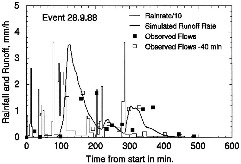
Fig. 7. Measured and simulated runoff for event of 28.9.88. Note that approximately 40 min change in time makes for an excellent match with the simulated flows.
