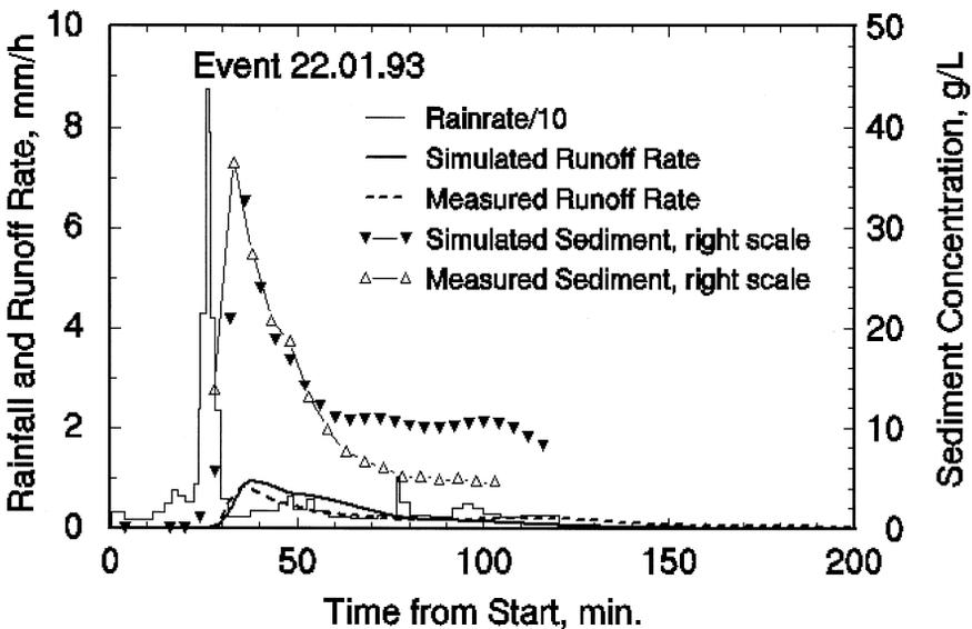
Fig. 10. Measured and simulated runoff for event of 22.1.93. There is an order of magnitude increase in the scale of 1993 sediment concentrations, compared with the 1987 events.
