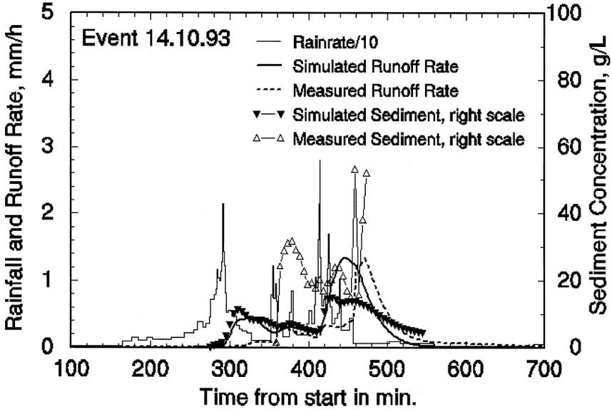
Fig. 12. Measured and simulated runoff for event of 14.10.93.
