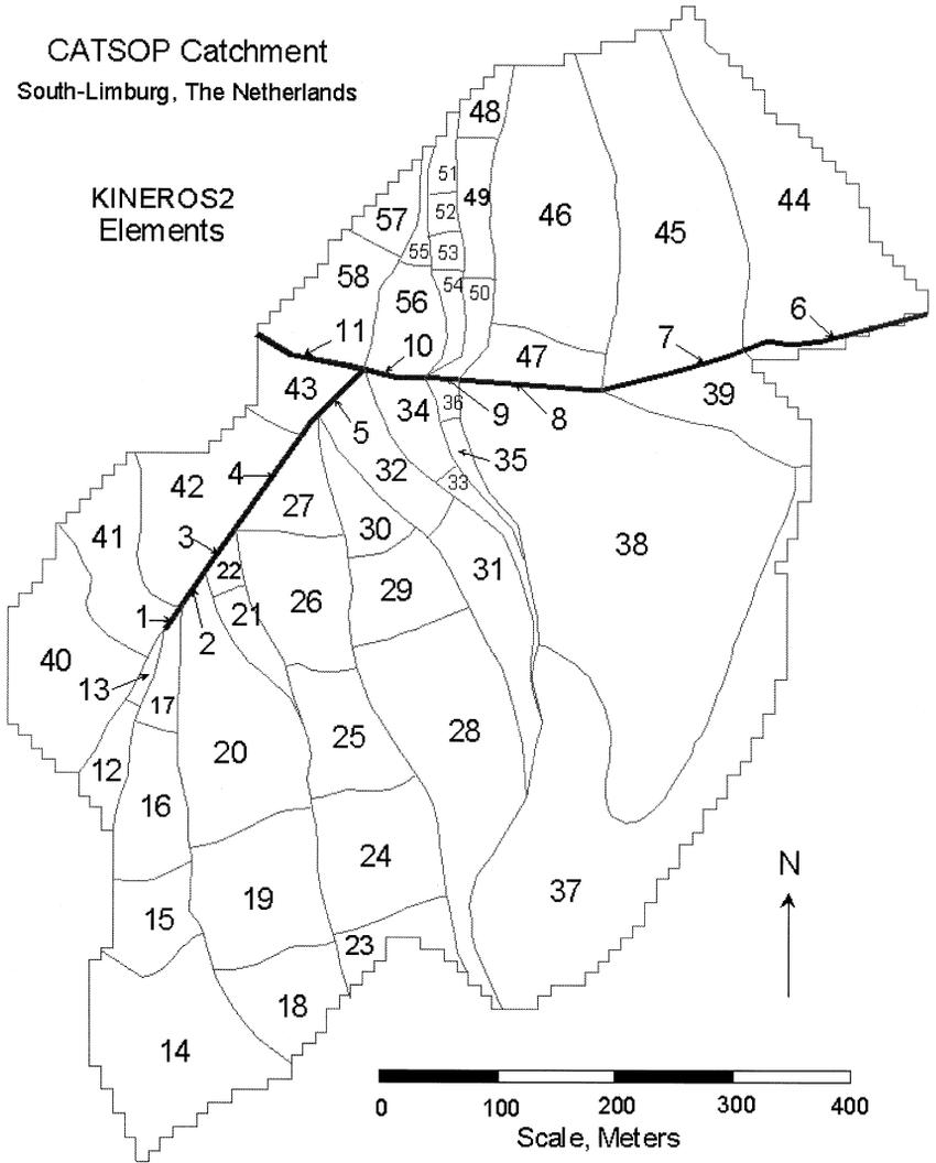
Fig. 2. Literal boundaries of the elements into which the Catsop catchment was subdivided for KINEROS2. It was assumed, in the absence of detail on furrow depth and direction, that flow follows topographic directions. Other subdivision were made to preserve management units.
