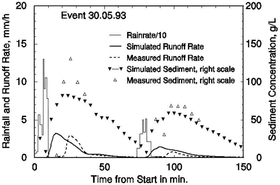
Fig. 11. Measured and simulated runoff for event of 30.5.93.
