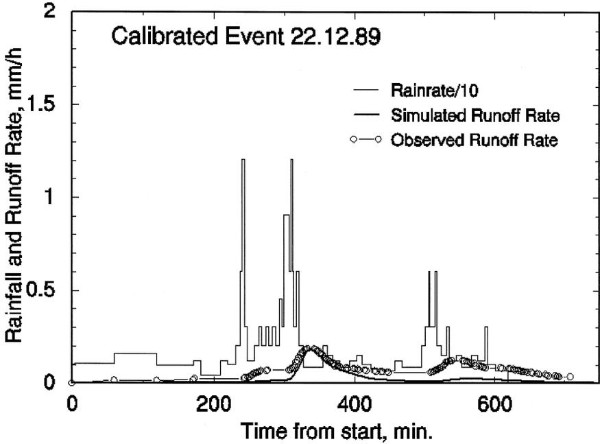
Fig. 5. Calibrated simulation of wet winter storm on 22.12.89.
