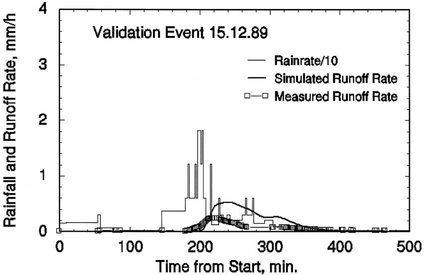
Fig. 6. Simulation of wet winter storm of 15.12.89 using parameters calibrated from event shown in Fig. 5. Both events apparently include interflow components for which KINEROS2 is not suited.
