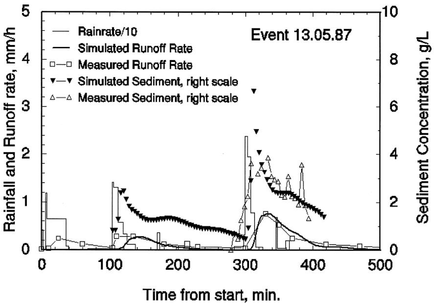
Fig. 8. Measured and simulated runoff for event of 13.5.87.
