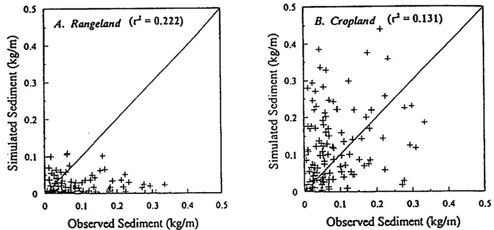
Figure 1. Comparison of observed sediment yield and WEPP model estimated sediment yield using the rangeland interrill erodibility adjustment factors (1a) and cropland interrill erodibility adjustment factors (1b).
