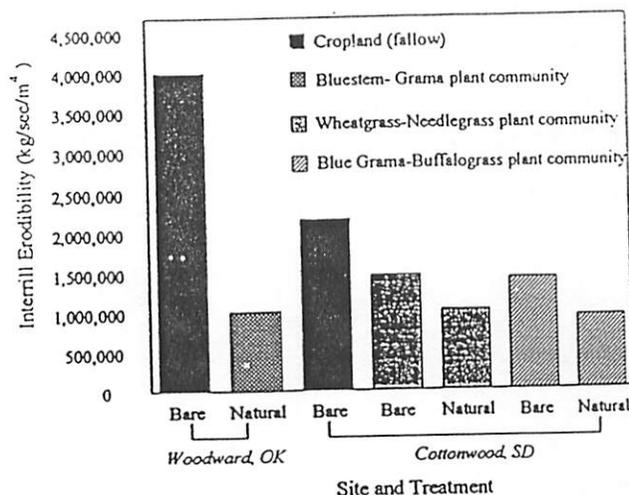
Figure 3 Comparison of fallow cropland and natural and recently bared rangeland soil interrill erodibilities on comparable phases of a soil series at two locations (from Lafren et al. 1991).
