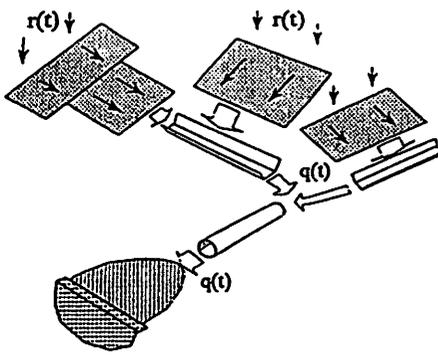
Figure 2. Schematic illustration of the major types of hydrologic elements in KINEROS2 and EUROSEM, and some of the ways that they may be arranged to simulate a complex watershed
