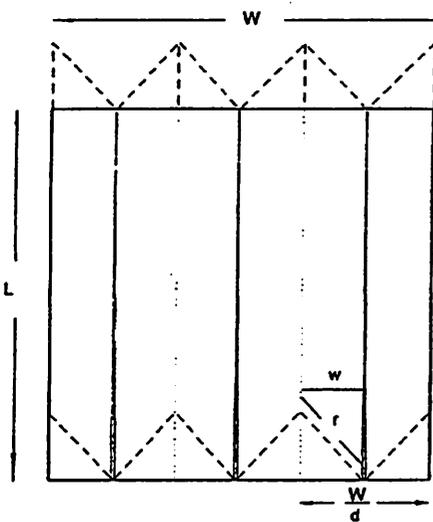
Figure 3. Diagram of the geometric approximation for rills used in EUROSEM
