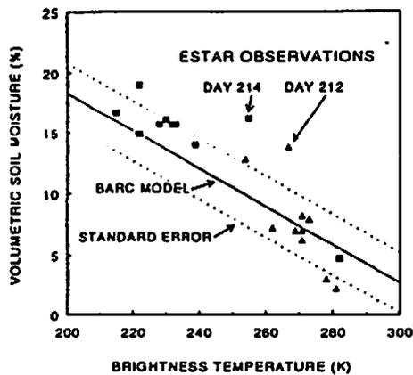
Figure 3. Observed and predicted relationships of soil moisture and ESTAR brightness temperature. BARC model based on ref. 8.
