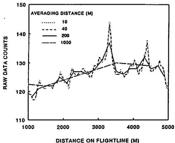
Figure 2. Effects of distance averaging on radiometer data patterns for L band.
