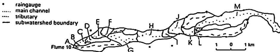
Fig. 2 Subwatershed 10 on Walnut Gulch Experimental Watershed showing channel system and subwatershed discretization for the distributed hydrologic model.
