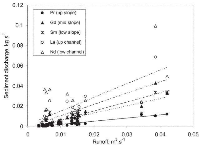
Fig. 5. Relationship between runoff and sediment rates from different morphological units of the watershed.
