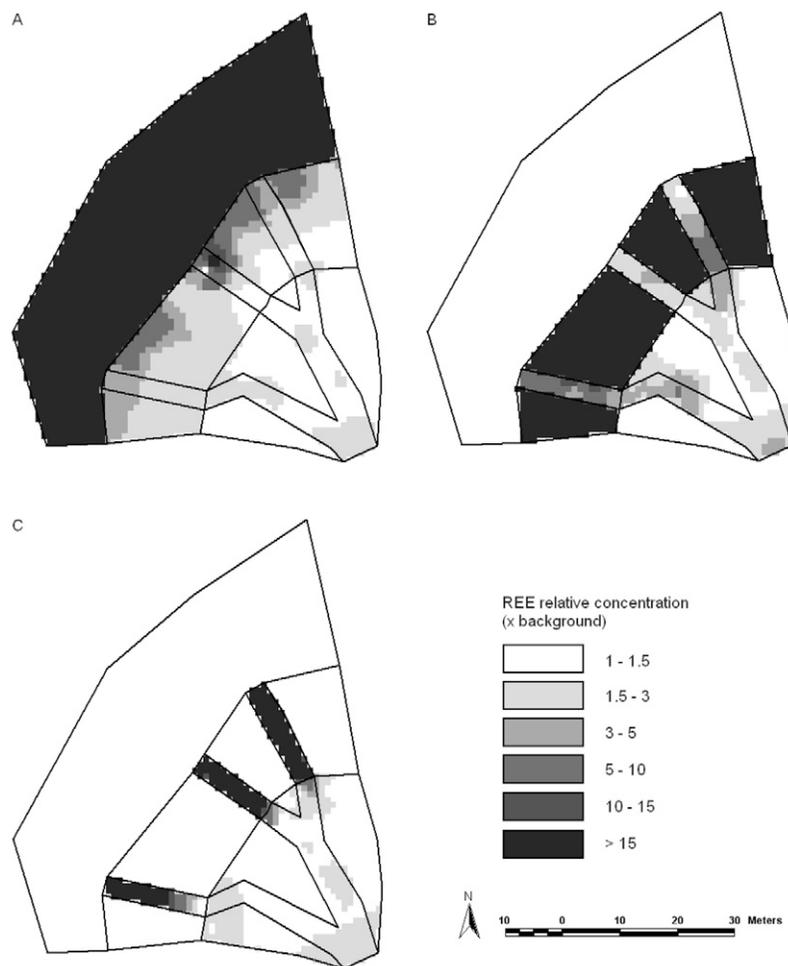
Fig. 4. Redistribution and pathways of rare earth element tracers in surface soil from upper slope (A), middle slope (B), and upper channel (C) by the end of the experimental period.
