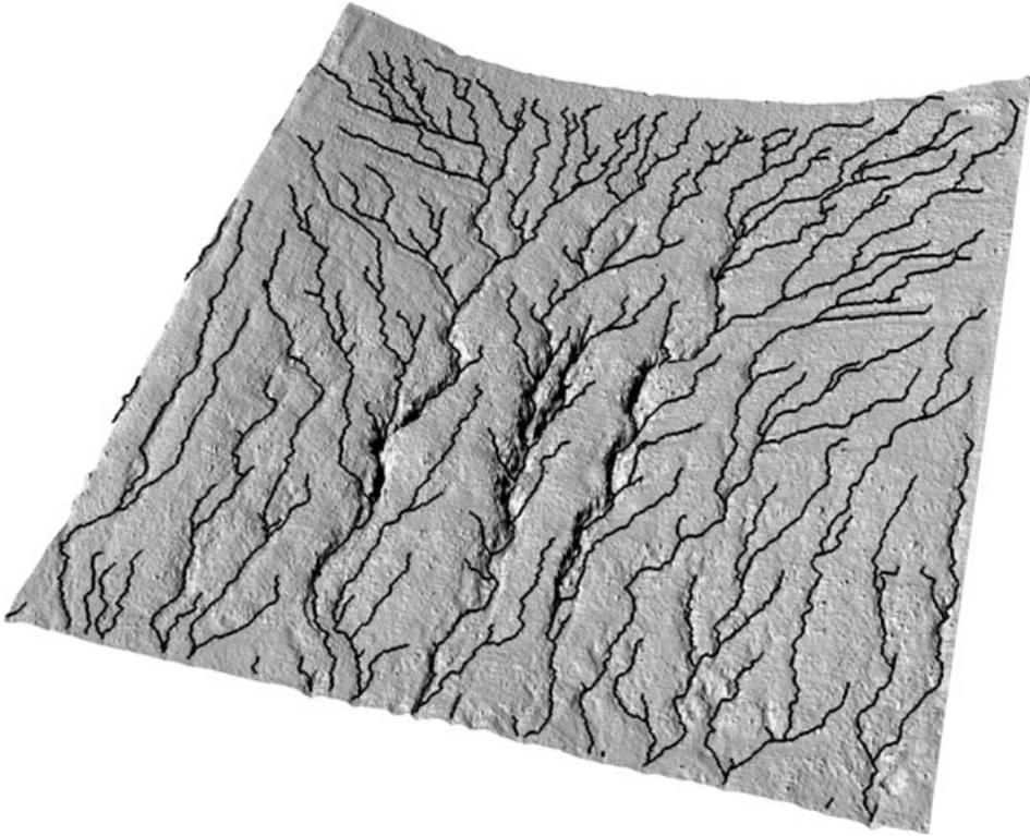
FIG. 8. A hillshading model of one soil surface DEM, three times exaggerated in Z. The rill network that developed on the surface was generated from the DEM and overlain on top of the DEM.
