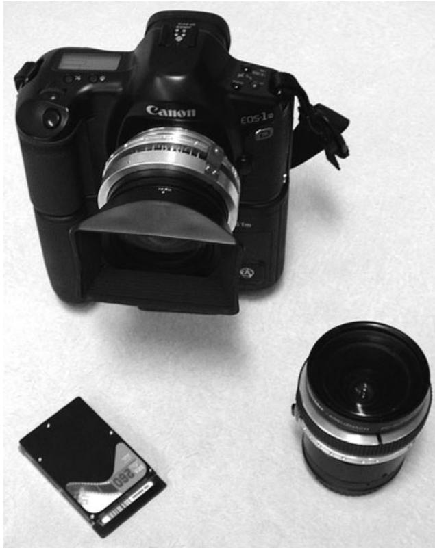
FIG. 2. Kodak DCS1m with Leica 19 mm lens mounted and Schneider 28 mm lens in the foreground. Images are saved on PCMCIA cards. Metal rings were fitted around both lenses to fix the focus distance and allow calibration for different reproducible distance settings.
