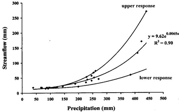
Figure 3 also includes two additional curves that were constructed to designate the lower and upper streamflow responses that would be expected to occur for a given amount of precipitation. Equation (1) was used to estimate the streamflow response that would be expected to occur for a given precipitation amount corresponding to a particular probability of exceedance.
