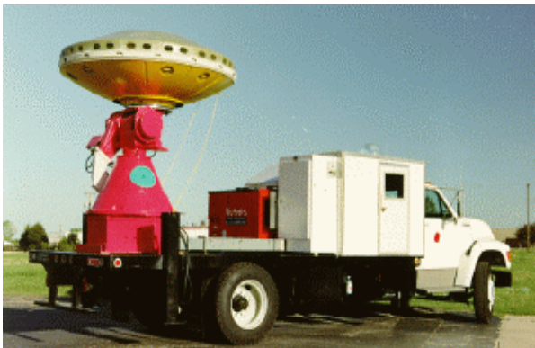
Figure 3. Doppler-on-Wheels (DOW) radar of the University of Oklahoma (deployment site marked by rectangle at upper end of catchment in Figure 1).
