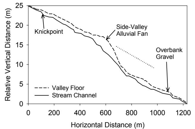
Figure 2. Typical longitudinal profile of an axial stream influenced by side-valley alluvial fans (modified from Miller et al. 2001).
