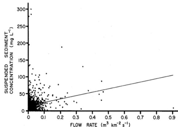
Figure 3. Suspended sediment concentration vs. per unit area flow rate.
