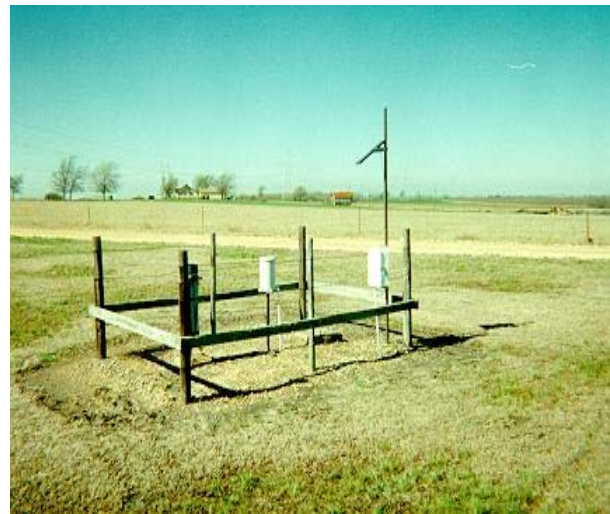
Figure 4. Recording tipping bucket rain gauge and datalogger setup with adjacent standard rain gauge.
