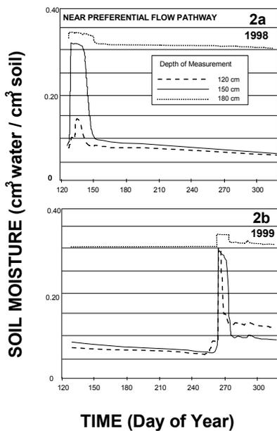
Figure 2. Real-time soil moisture observations near the GPR-identified flow pathway.
