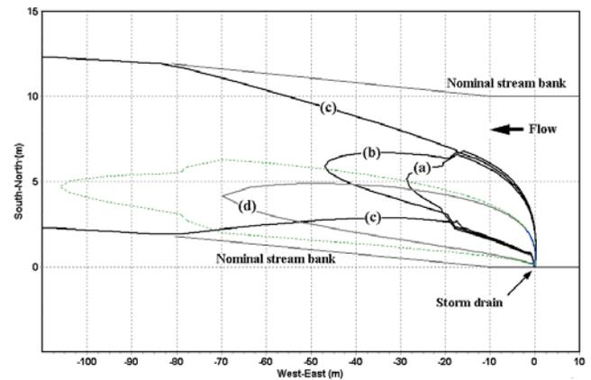
Figure 4. Simulated plumes--solid isopleths define the  $100 \text{ ng/L}$  ambient diazinon criterion concentration. Storm drain flows are (a)  $0.233$ , (b)  $0.243$ , (c)  $0.253$ , and (d)  $0.116 \text{ m}^3 \text{ s}^{-1}$ , respectively. The light dashed isopleth,  $95 \text{ ng/L}$  concentration, part of Plume (d), shows how concentrations further decrease under these conditions.
