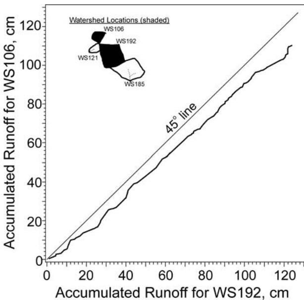
Figure 7. Double-mass plot of monthly runoff between WS106 and WS192.
