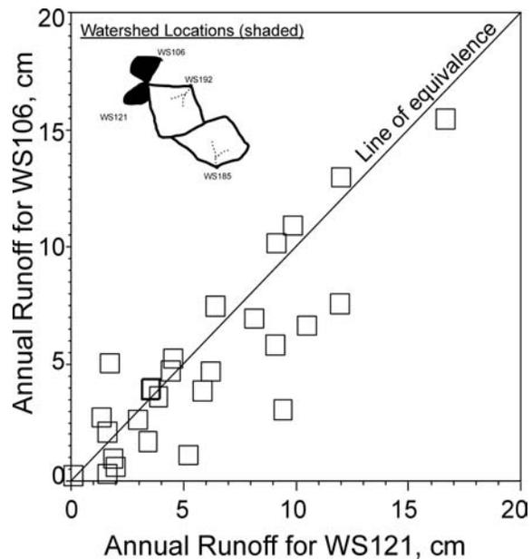
Figure 4. Annual runoff comparison between WS106 and WS121.
