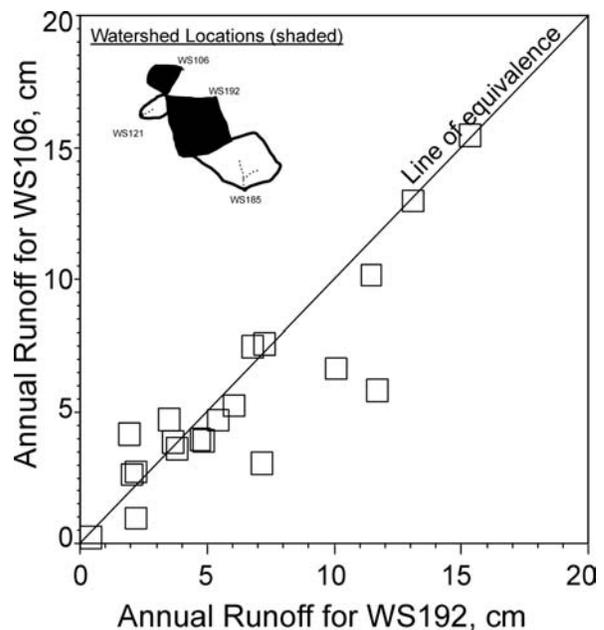
Figure 5. Annual runoff comparison between WS106 and WS192.
