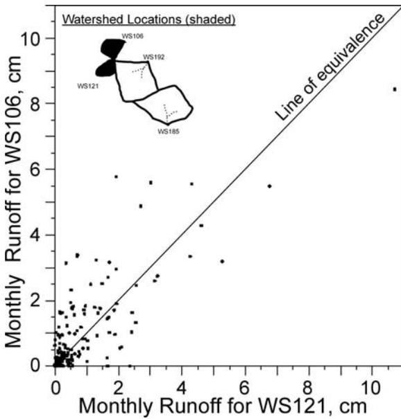
Figure 6. Monthly runoff comparison between WS106 and WS121.
