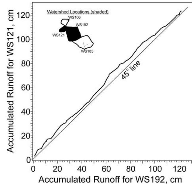
Figure 8. Double-mass plot of monthly runoff between WS121 and WS192.
