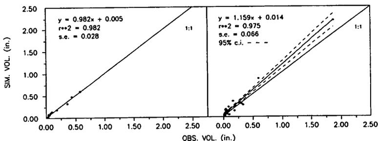
Figure 1a. Simulated versus observed runoff volumes for pretreatment period (1973-80) optimization events for LH106.
