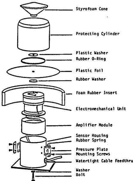
FIGURE 1. Exploded view of the transducer (after Joss and Waldvogel, 1970)
