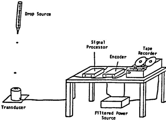
FIGURE 2. Static drop calibration configuration.
